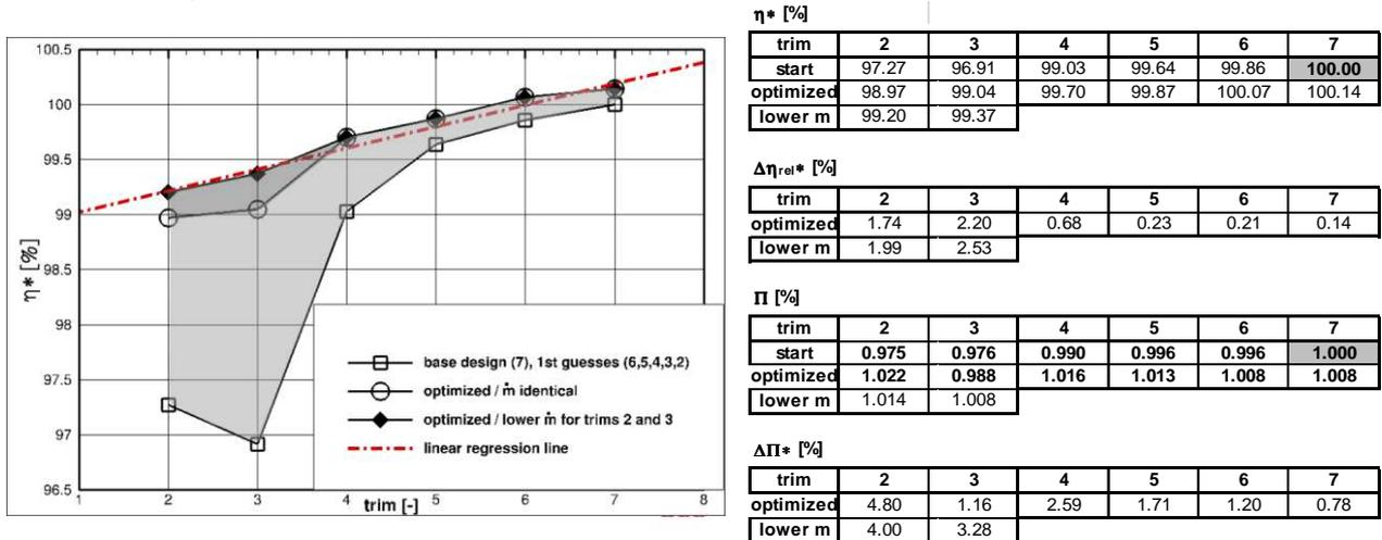
**Fig 6: Efficiency Gain per Trim Optimization**      **Table 1: Efficiency and Pressure Ratio per Trim Optimization**
