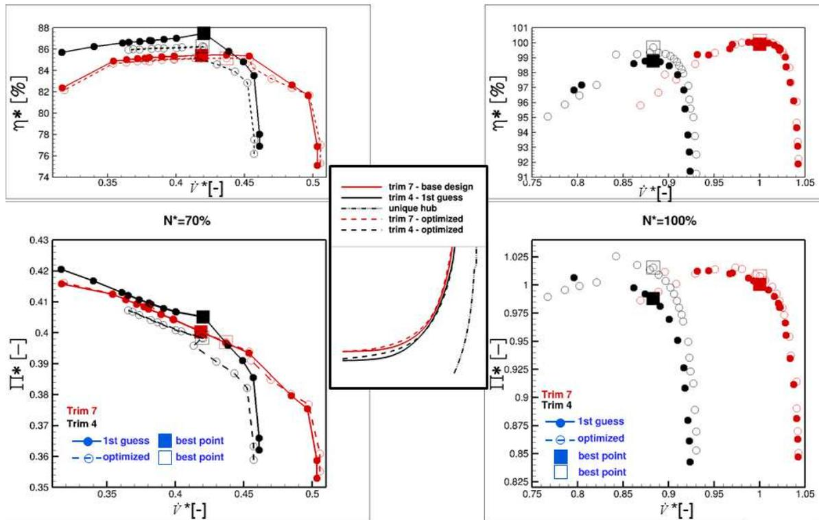
Figure 7: Compressor Map – Off-Design Speed (left)– Design Speed (right)
