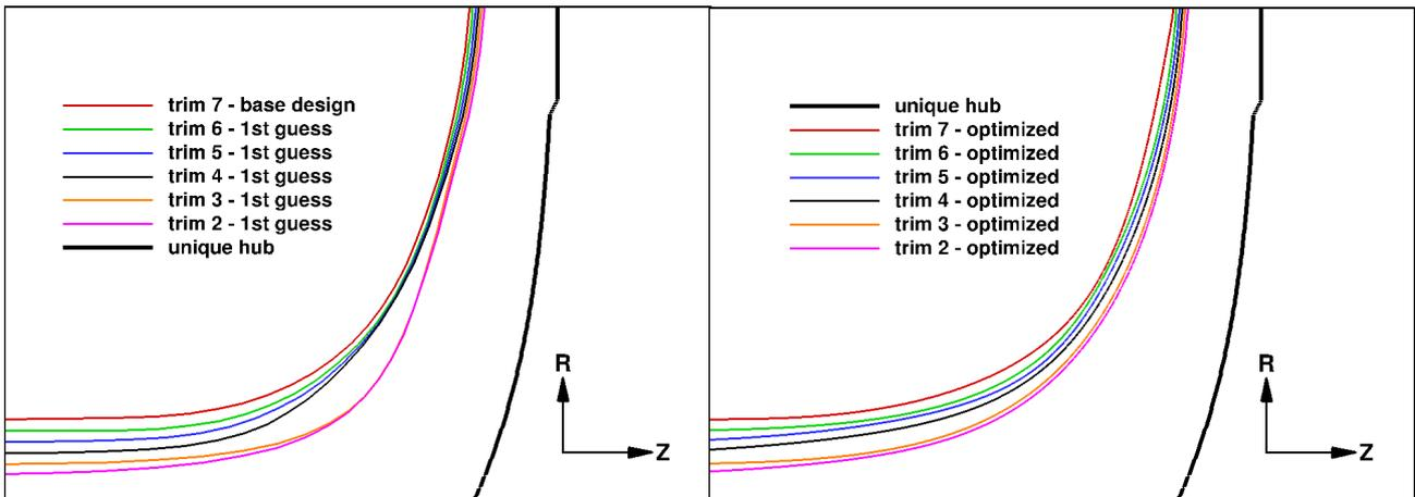
**Figure 5: Shroud Contours: First Guesses (left) and optimized (right)**
