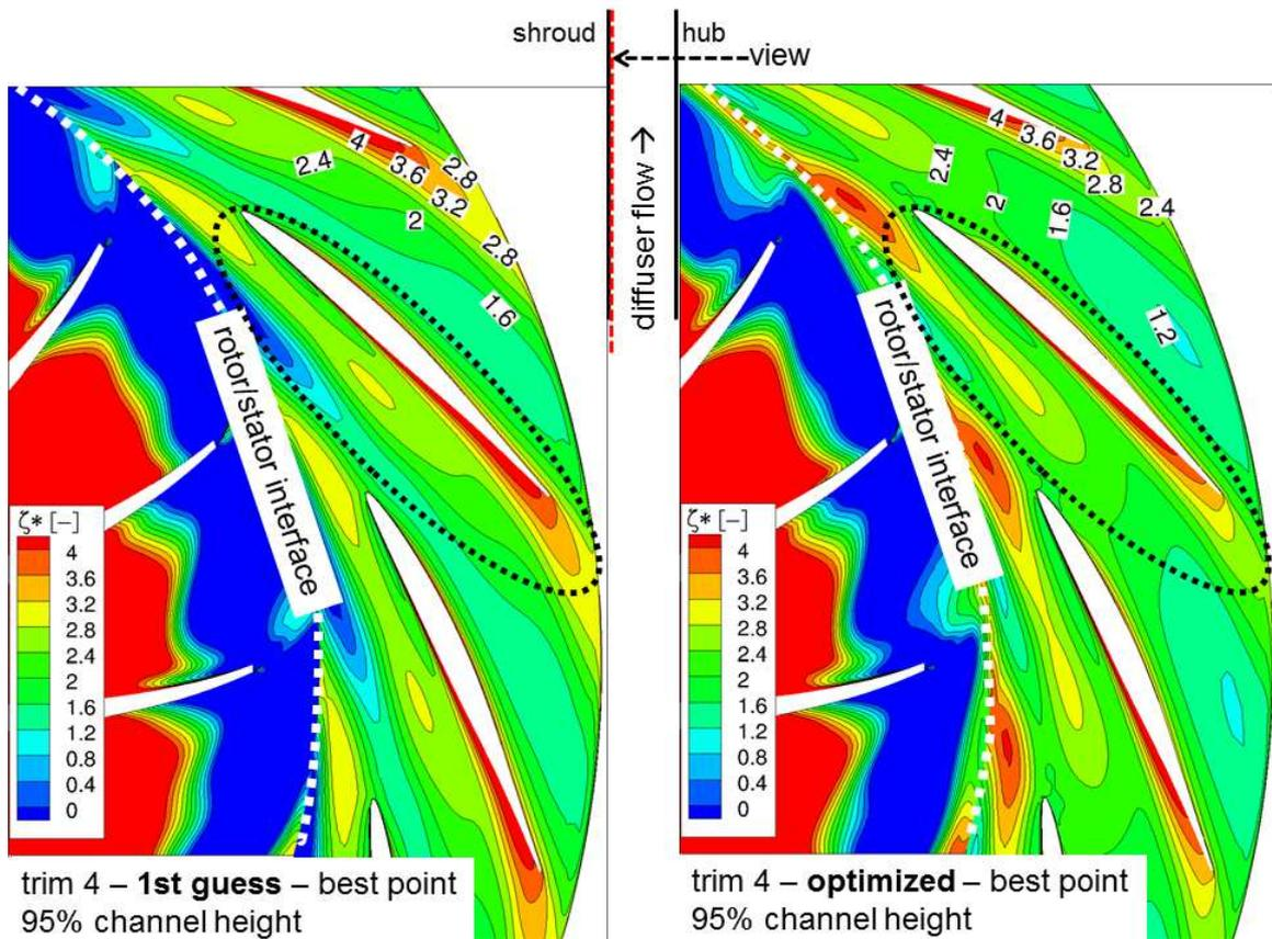
Figure 9: Diffuser: Total Pressure Loss Coefficient at 95% Channel Height
