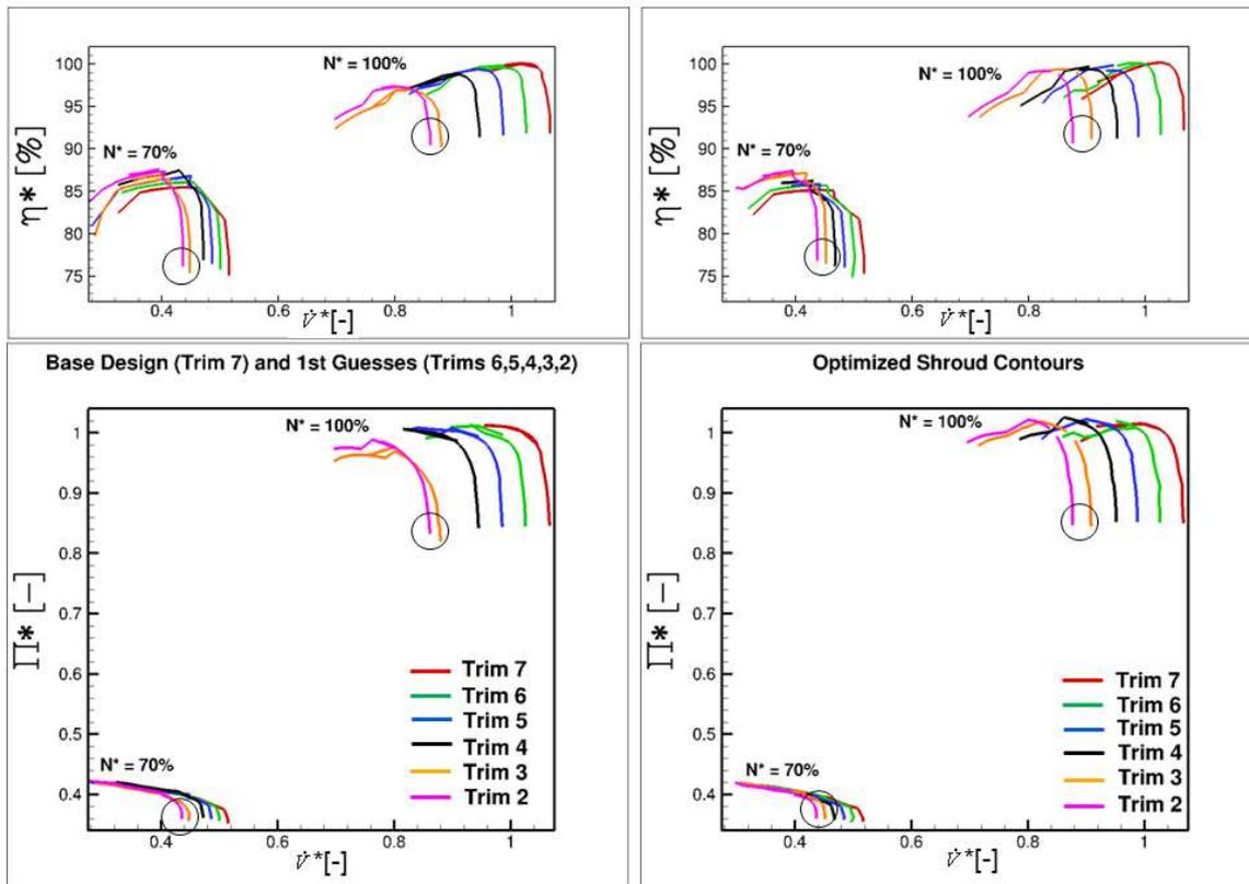
Figure 10: Set of 2 Speed Lines – Base Design+1<sup>st</sup> Guesses (left) – Optimized (right)
