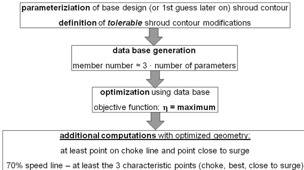
**Figure 4: Flow Chart of the Optimization Process**
