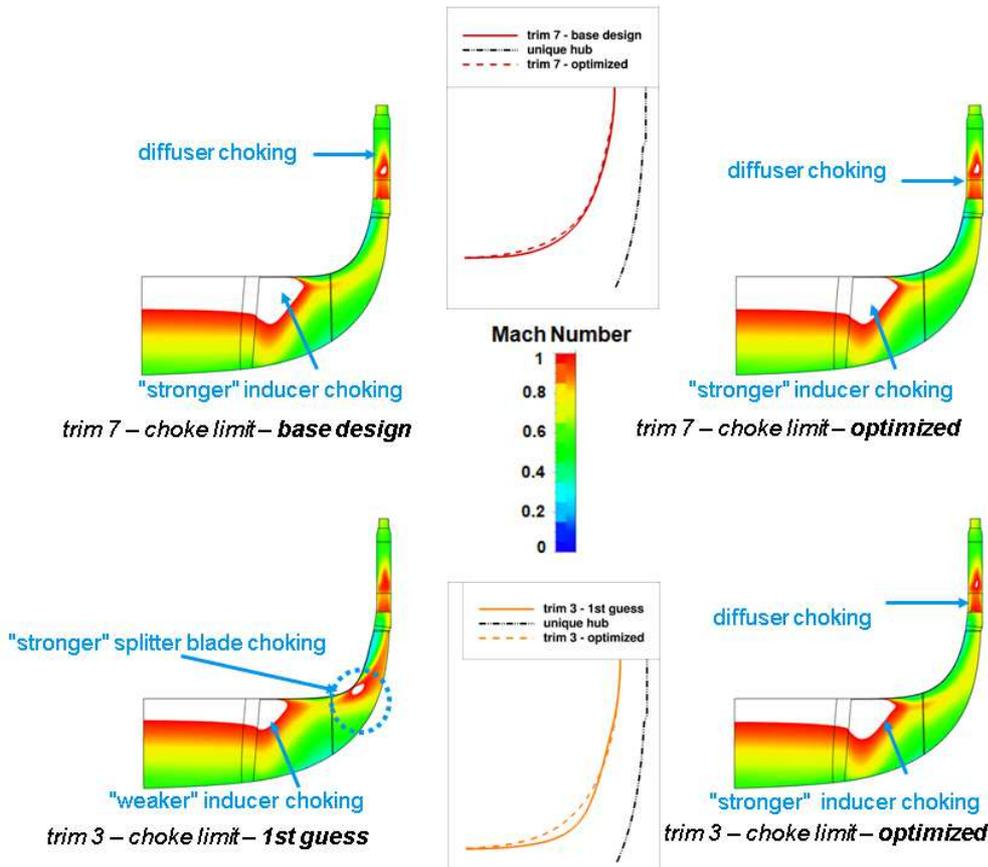
Fig 11: Corresponding Operating Points on Choking Line for Trims 7 and 3 – for start and optimized Shroud Contours, circumferentially averaged Mach number in Meridional Plane
