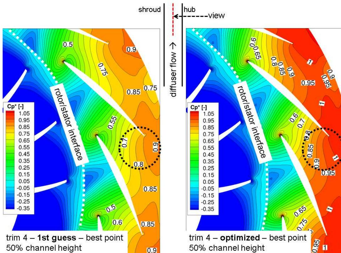
Figure 8: Diffuser: Pressure Recovery Coefficient at 50% Channel Height
