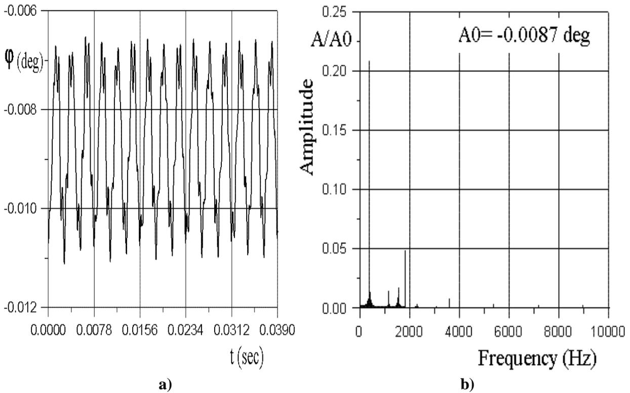
**Figure 5: Amplitude-frequency spectrum of R1 blade torsional oscillations (peripheral layer), unblocked inlet**
