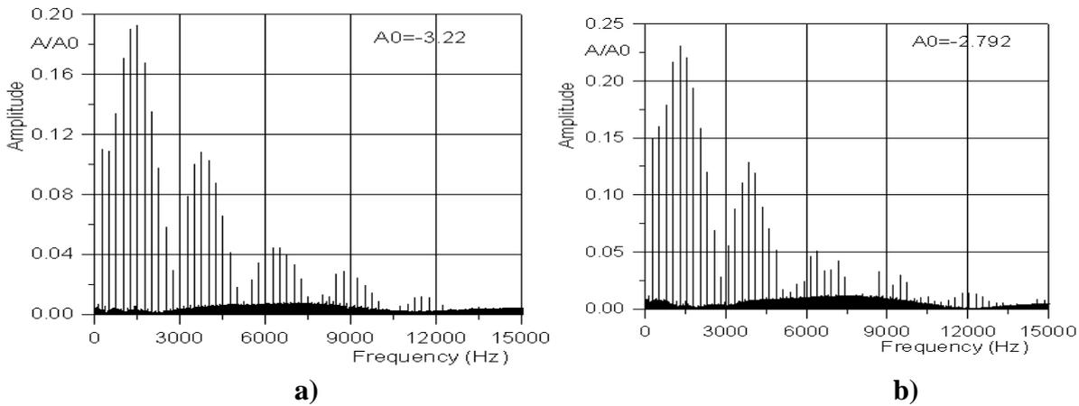
**Figure 2: Amplitude frequency spectrum circumferential  $F_y$  and axial force  $F_z$  for the peripheral layer of R1 blade**
