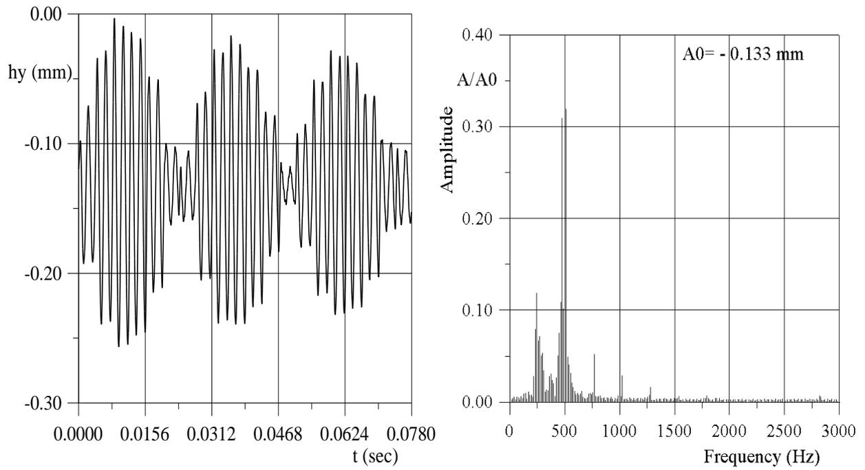
**Figure 7a: R2 blade displacement (peripheral layer, circumferential direction  $h_y$ , blocked inlet)**
