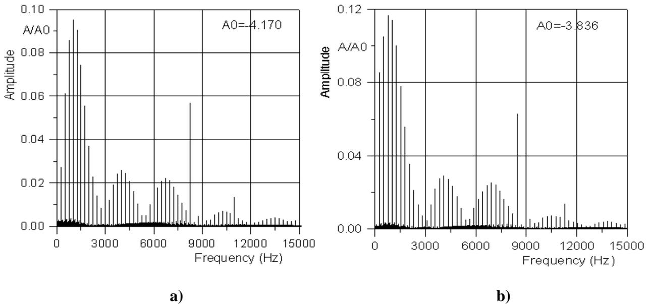
**Figure 3: Amplitude frequency spectrum circumferential  $F_y$  and axial force  $F_z$  for the peripheral layer of R2 blade**
