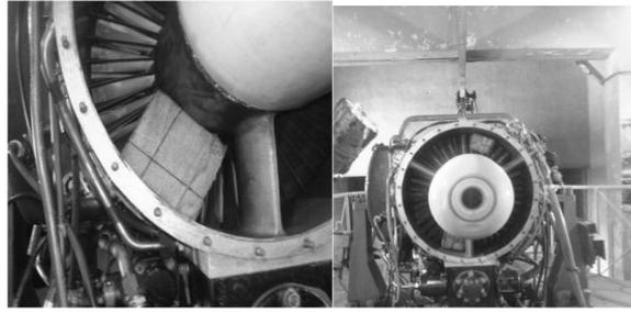
**Figure 1a: Test rig of SO-3 engine**
