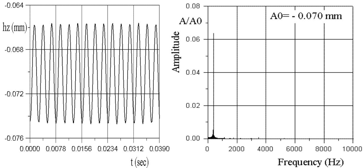
**Figure 4a: R1 blade displacement (peripheral layer, axial direction hz), unblocked inlet**
