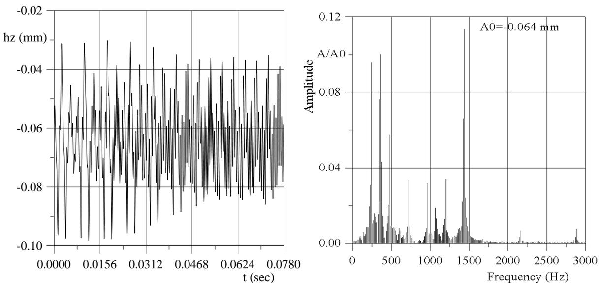
**Figure 4b: R1 blade displacement (peripheral layer, axial direction hz), blocked inlet**
