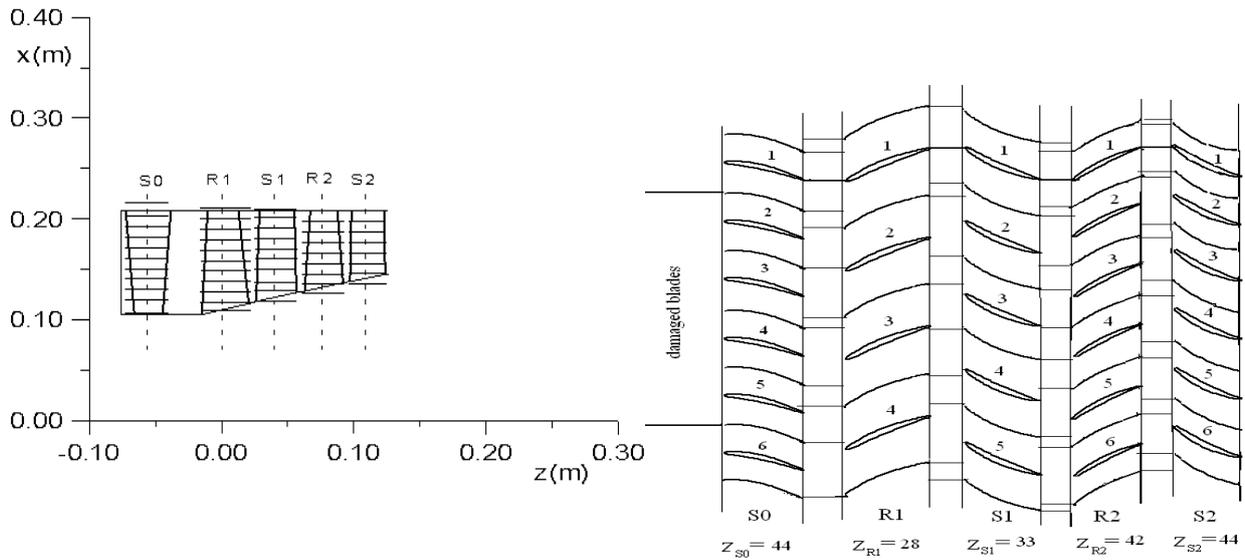
**Figure 1b: Computational model of the 2.5 stage (S0-R1-S1-R2-S2)**
