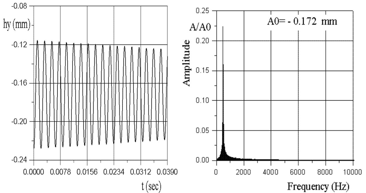
**Figure 7b: R2 blade displacement (peripheral layer, circumferential direction  $h_y$ , unblocked inlet)**
