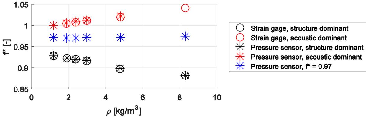
Figure 10: Overview of the resonance frequencies of the considered modes.
