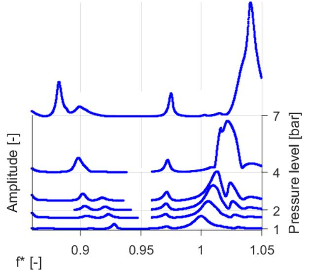
Figure 9: STFT results of frequency sweeps at different pressures (pressure sensor data).
