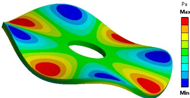
**Figure 5: Structure dominant (in-phase) mode with four nodal diameters and zero nodal circles. The disk is displayed with the acoustic pressure pattern. Result of the numerical modal analysis.**
