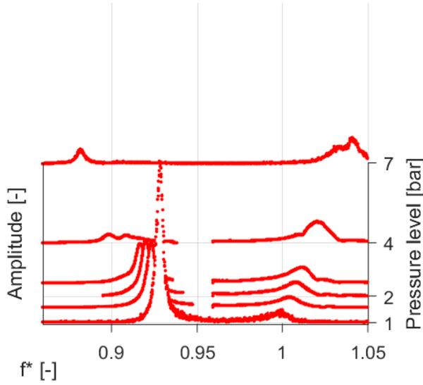
Figure 8: STFT results of frequency sweeps at different pressures (strain gage data).
