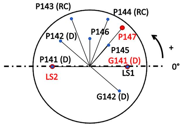
**Figure 4: Normal view of the rotor-stator test rig with the sensors' allocation. Within this paper results of the red marked sensors are presented. Labels: "P": pressure sensor, "G": strain gage, "LS": loudspeaker, "RC": rear cavity, "D": disk**
