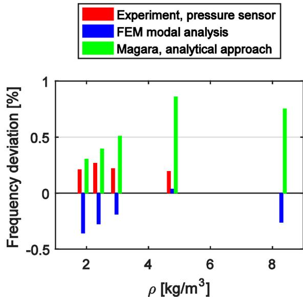
**Figure 14: The relative resonance frequency deviation of the different results to the strain gage data. Acoustic dominant mode.**
