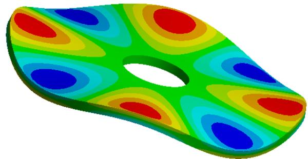
**Figure 6: Acoustic dominant (out-of-phase) mode with four nodal diameters and zero nodal circles. The disk is displayed with the acoustic pressure pattern. Result of the numerical modal analysis.**
