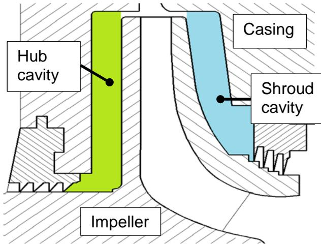
**Figure 1: A meridional sketch of a radial compressor stage with the side cavities.**
