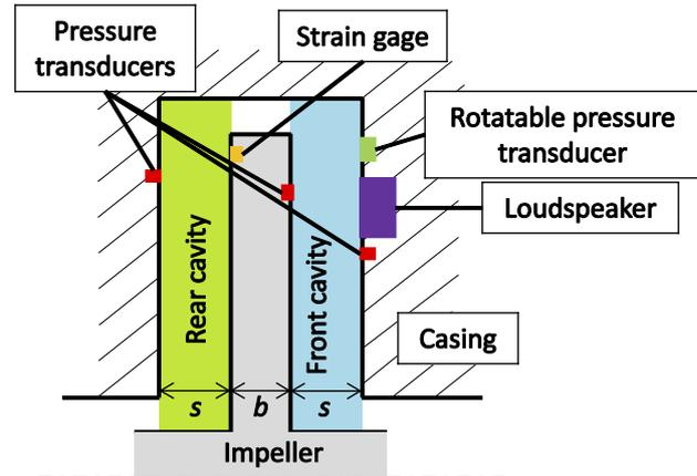
**Figure 2: Sketch of the rotor-stator test rig with the acoustic specific instrumentation (meridional view).**
