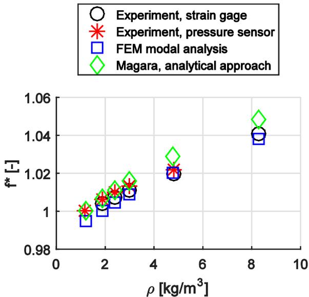
**Figure 13: The resonance frequency of the acoustic dominant mode at different gas densities. Comparison of different results.**
