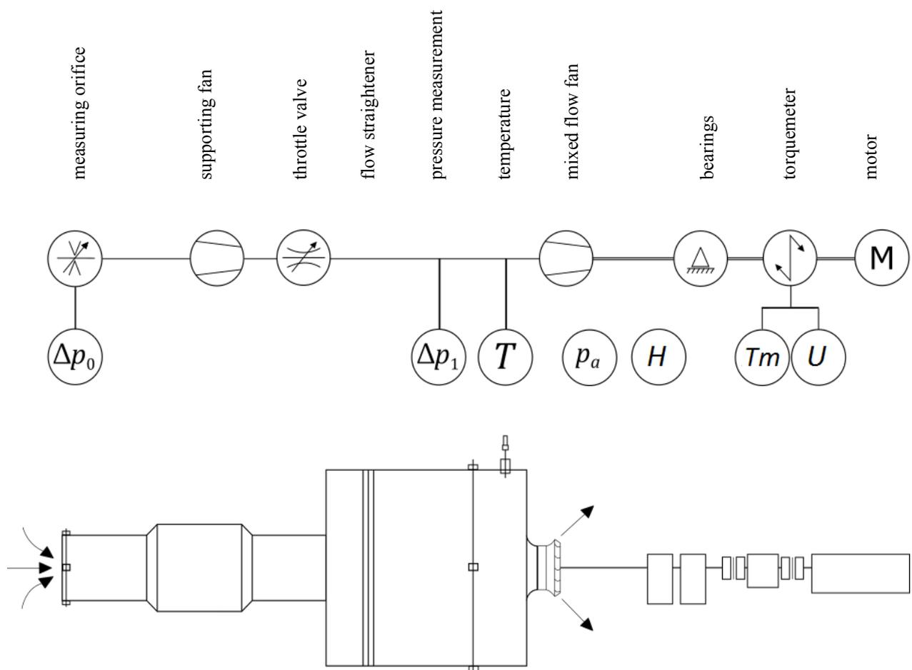
**Figure 2: Ventilator test stand corresponding to EN ISO 5801, located at the Fluid System Dynamics Department at the Technical University of Berlin**
