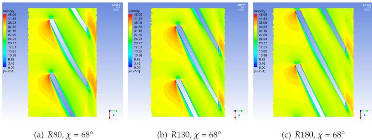
**Figure 7a-c: blade to blade sections for mixed flow fans of radii R80, R130 and R180**
