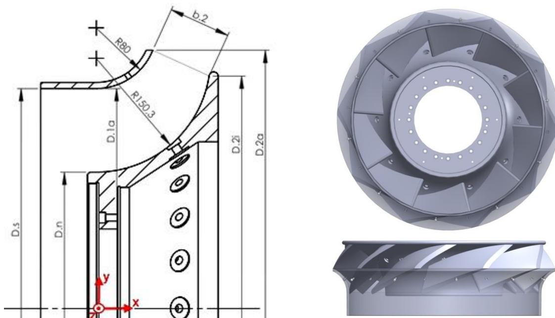
**Figure 1: Hub and shroud contour of a mixed flow fan with a shroud radius of R80 (left) and ten backward curved constant thickness blades, installed in the mixed flow fan, adapted from the radial “Pfleiderer” blade design method**
