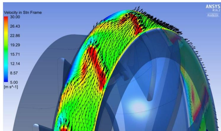
**Figure 3: Flow separation on the shroud of a mixed flow fan with radius R80 and downstream angle  $\chi = 68^\circ$**
