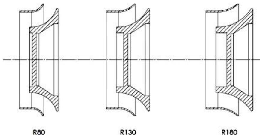
**Figure 4: Modified shroud of a mixed flow fan with 3 different radii (R80, R130 and R180)**
