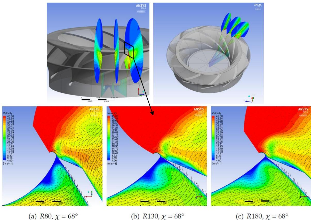
**Figure 6a-c: Vortex structure of flow separation on the shroud for mixed flow fans of various radii**
