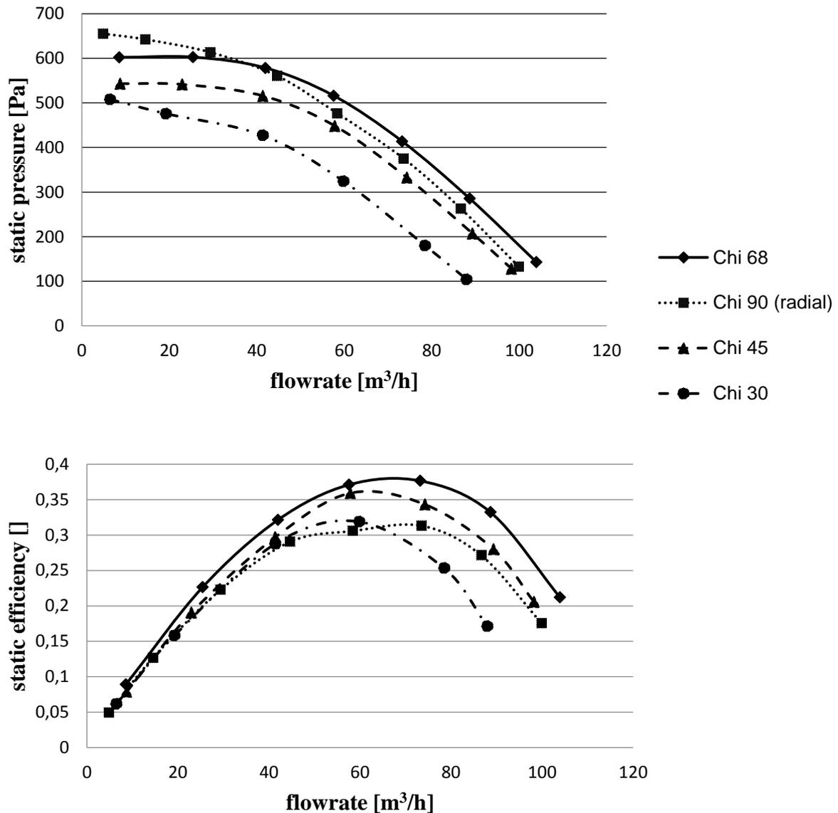
**Figure 9: measured characteristic curves of four different mixed flow fans with downstream angles of  $\chi = 30^\circ$  (dashed dotted line),  $\chi = 45^\circ$  (dashed line),  $\chi = 68^\circ$  (black line) and  $\chi = 90^\circ$  (dotted line)**
