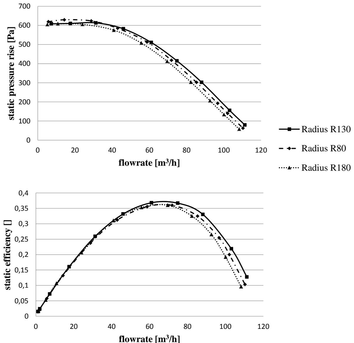
Figure 5: measured characteristic curves for three mixed flow fans with different shroud radii of R80, R130 and R180
