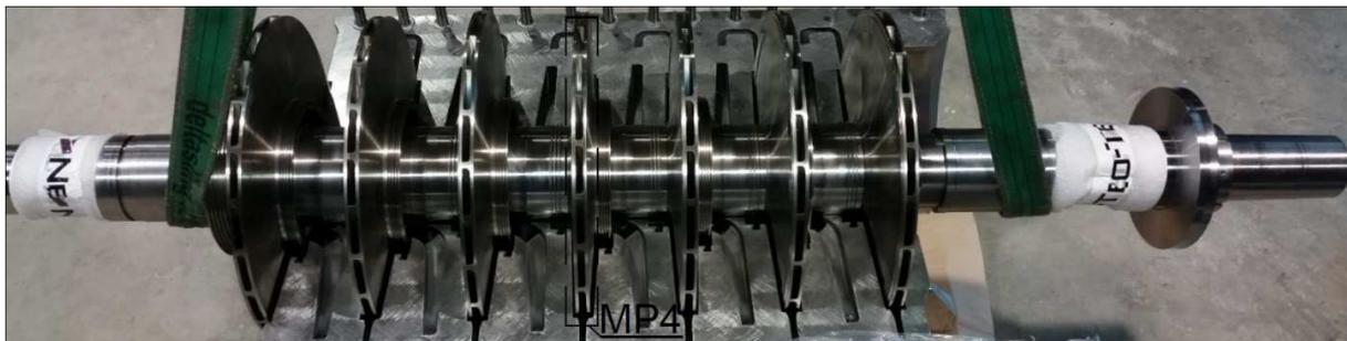
Figure 7: MP rotors of a modernized compressor and HP rotor during assembling
