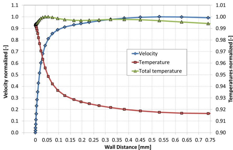
**Fig. 3 Profiles for velocity, static temperature and total temperature in the boundary layer**
