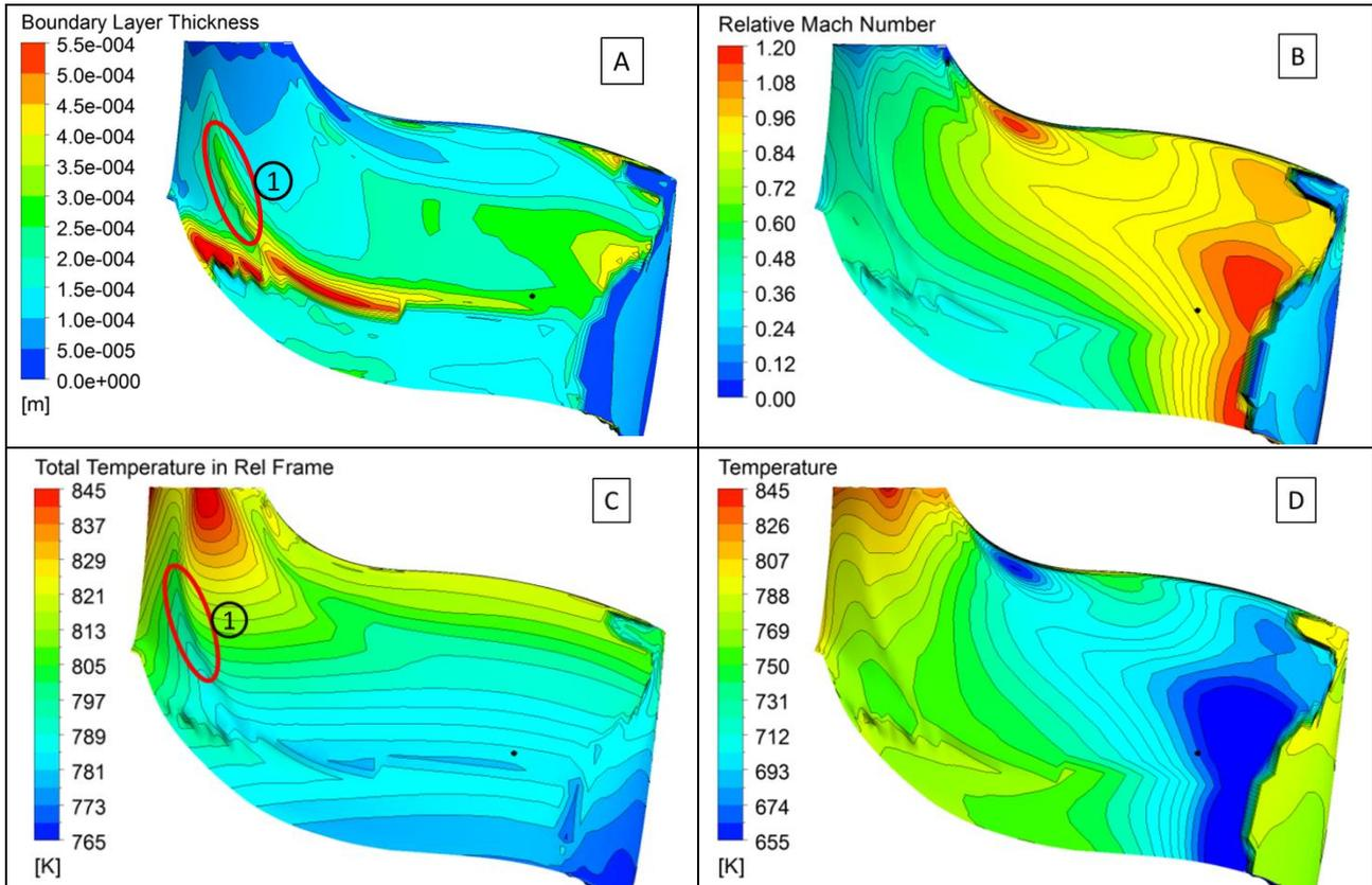
**Fig. 7** Aero-thermodynamic state at the edge of the boundary layer  $u = 1.0 u_0$ ,  $T_{\text{tot, TI}} = 873 \text{ K}$ ,  $\dot{m}_T = 0.96 \dot{m}_{T,0}$
