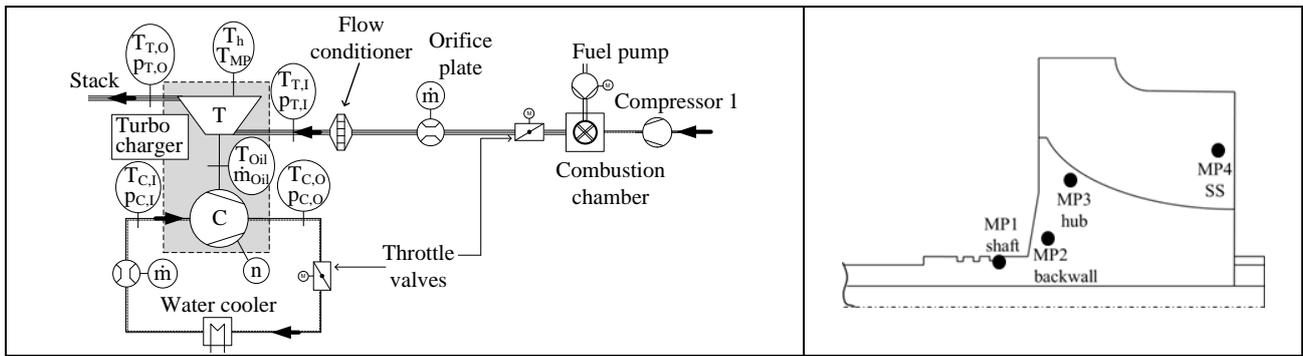
**Fig. 1 Scheme of the test rig for steady state operating points (left) and Position of the thermocouples at the turbine wheel (right)**
