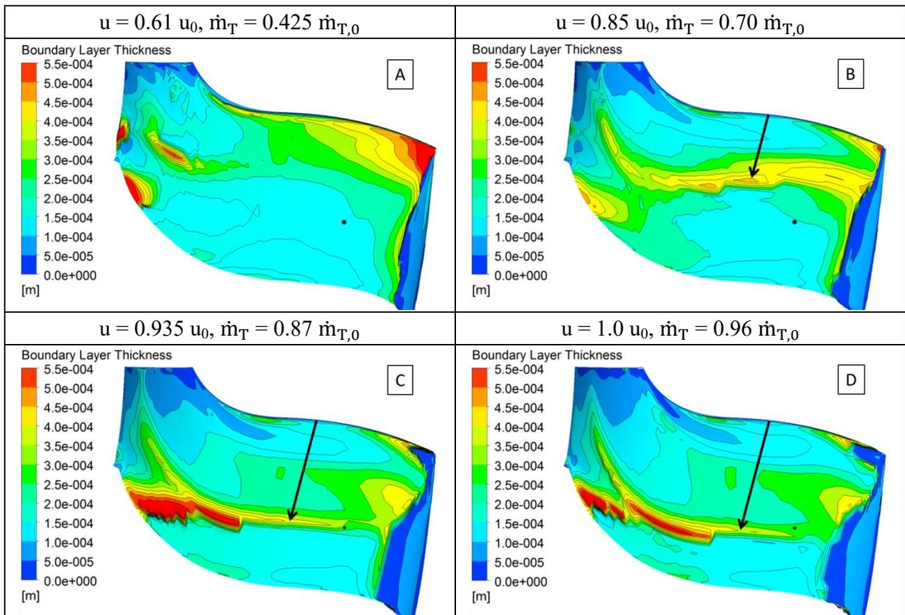
**Fig. 5 Boundary layer thickness at suction side for four operating points,  $T_{\text{tot,TI}} = 873 \text{ K}$**
