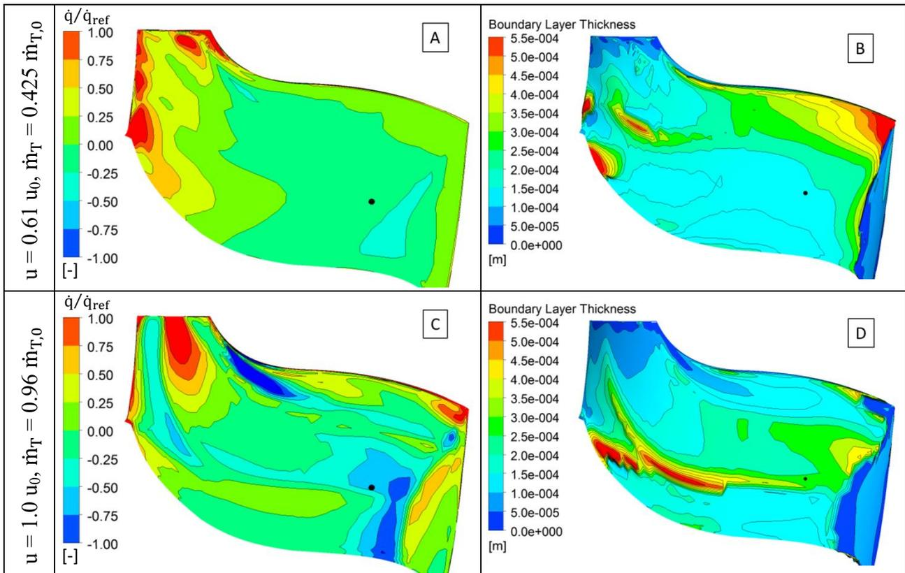
**Fig. 8 Comparison of Wall heat flux and boundary layer thickness at suction side for two operating points,  $T_{\text{tot, TI}} = 873 \text{ K}$**
