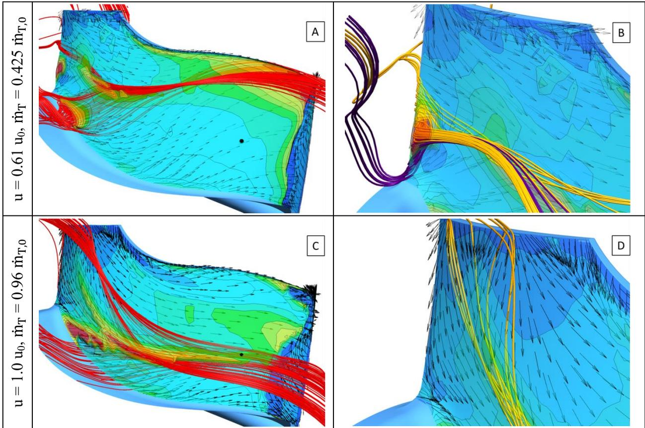
**Fig. 6 Secondary flow phenomena at suction side for two operating points,  $T_{\text{tot,TI}} = 873 \text{ K}$**
