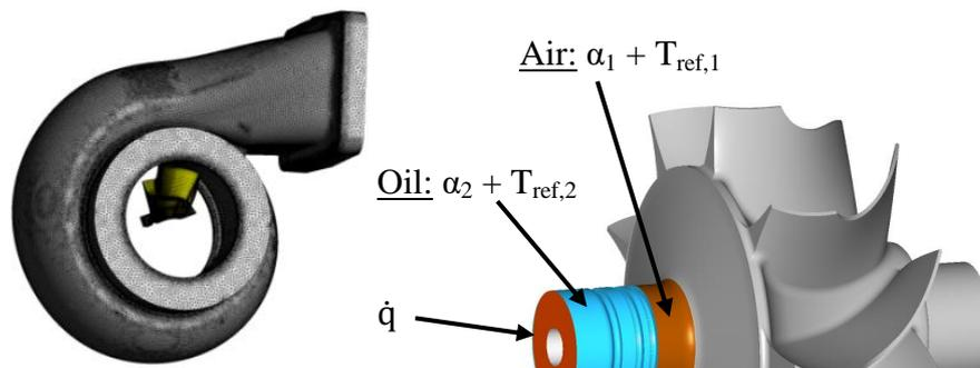
**Fig. 2 Numerical model without inlet and outlet pipes**
