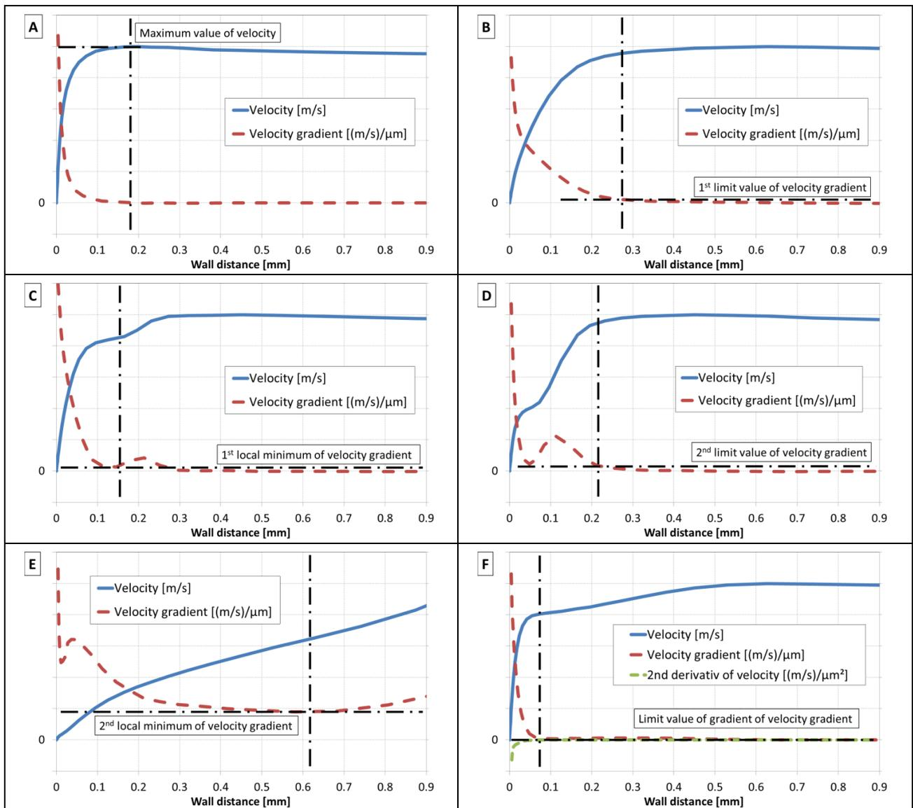
**Fig. 4** Defined criteria to evaluate the boundary layer thickness
