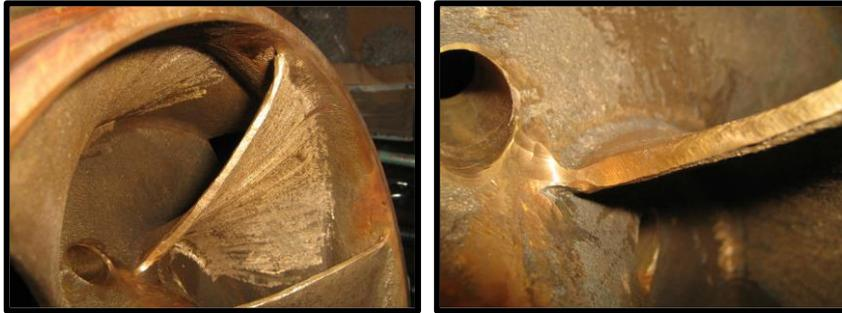
**Figure 3: Detail of the blade geometry – focus on the leading edge**
