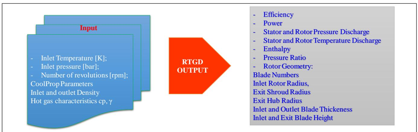
Figure 4: RTGD Diagram
