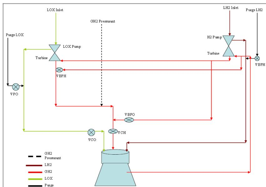
**Figure 3: Schematic of VINCI System [1]**
