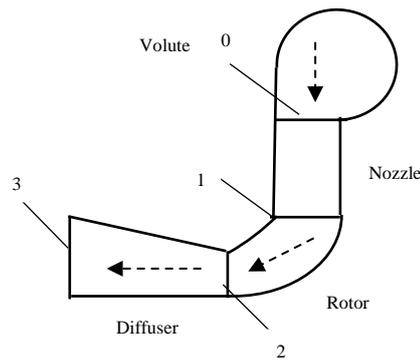
**Figure 1: Radial Turbine Stage Cross Section**
