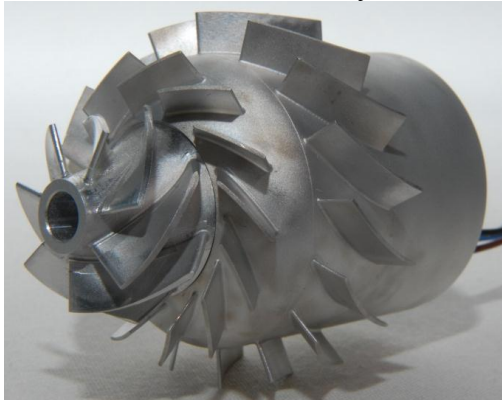
Figure 4: Prototype of compressor A, showing mixed flow impeller, vaned diffuser, axial de-swirl vanes and enclosed electric motor with a length of 85 mm, and overall diameter of 60 mm
