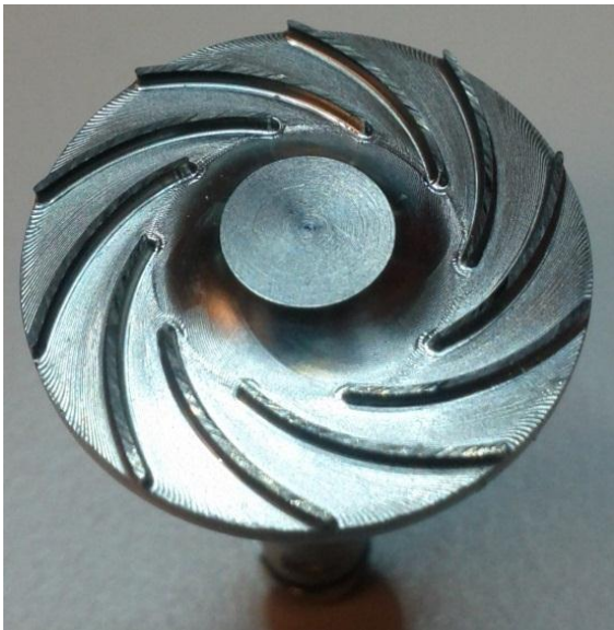
Figure 6: Impeller of compressor B, diameter: 21 mm, rotor length: 36 mm
