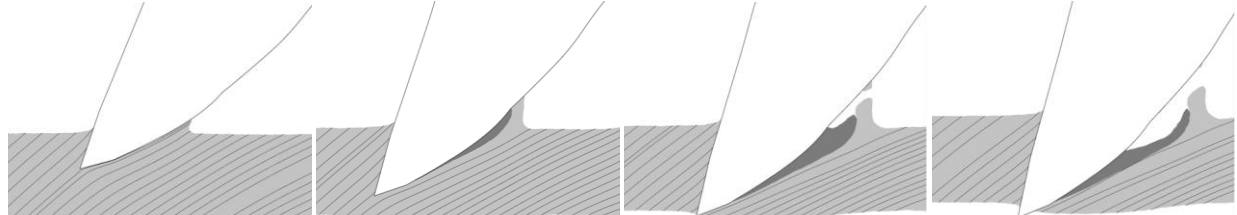
Fig. 9. Relative streamline on the symmetry plane, ■ water, ■ water vapour ( Q = 50\% Q_{Des} ).
