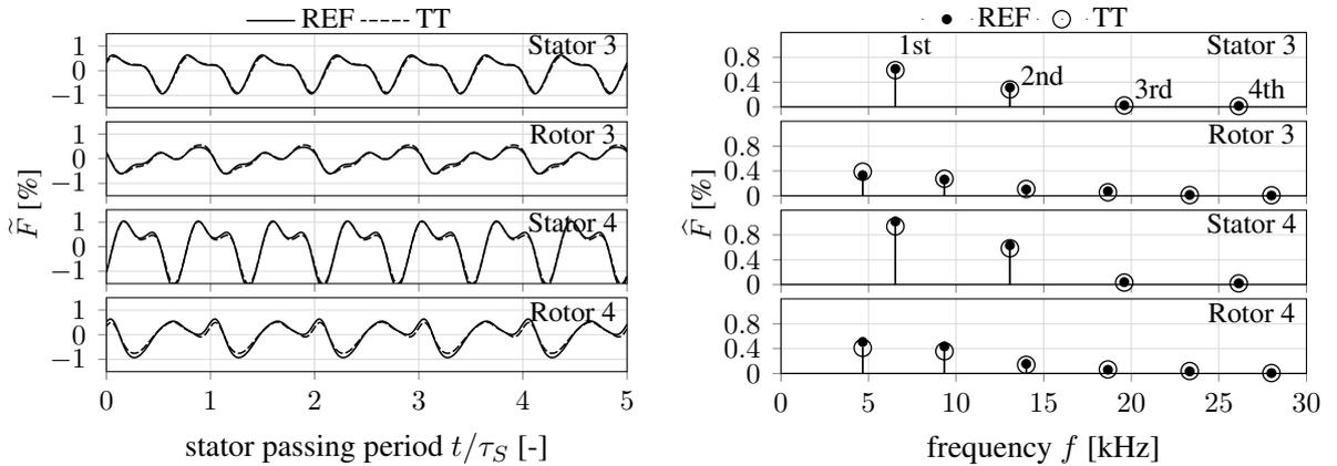
Fig. 6: Force fluctuations over stator passing period (left); Frequency spectra of the force signals (right)
