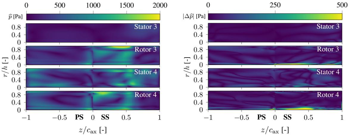
Fig. 7: **First harmonic amplitude of the pressure signal (REF) (left); absolute variance between REF and TT case (right)**
