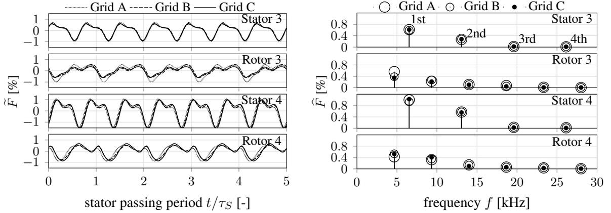
Fig. 5: Force fluctuations over stator passing period (left); Frequency spectra of the force signals (right)
