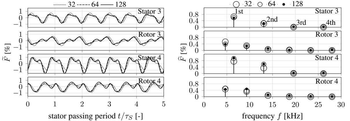
Fig. 4: **Force fluctuations over stator passing period (left); Frequency spectra of the force signals (right)**
