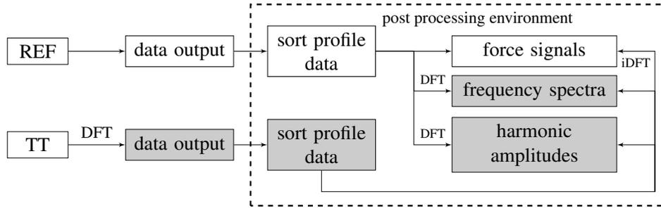
Fig. 3: **Process describing the post processing procedure; white: time domain data; grey: frequency domain data**
