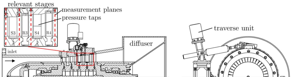
Fig. 1: Sectional views of the turbine test rig
