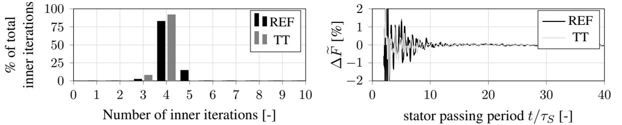
Fig. 9: Percentage of total inner iterations (left); Convergence of Rotor 3 force signal (right)
