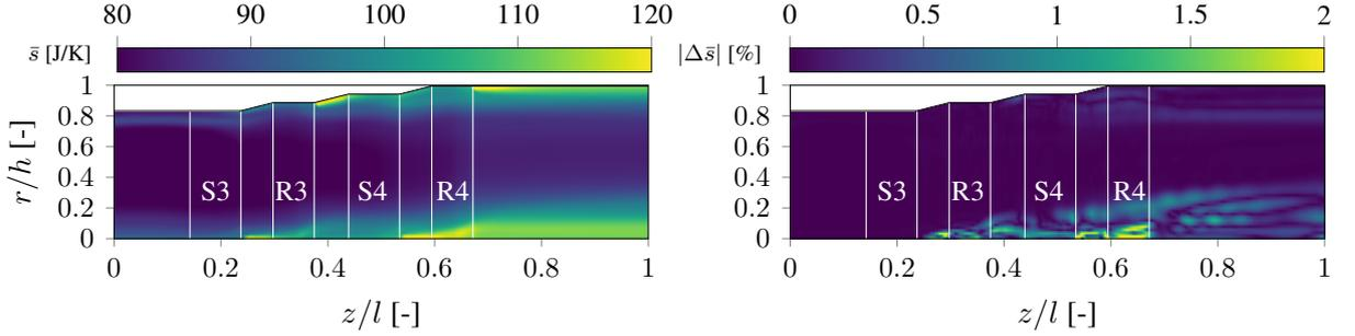
Fig. 8: Circ. averaged entropy  $\bar{s}$  for reference calculation (left); Percentage variance of  $\bar{s}$  (right)
