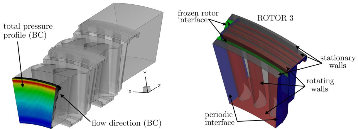
Fig. 2: **Computational domain with inlet distribution of total pressure BC and velocity vectors (left); Boundary conditions for one blade row (right)**
