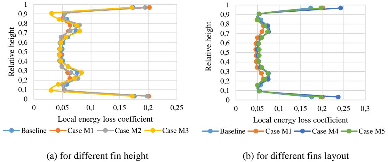
**Figure 5: Distribution of local energy loss coefficient along the height of studied vane model**
