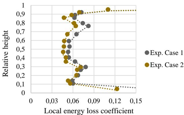
**Figure 10: Distribution of local energy loss coefficient along the height of vane model obtained during experiments**
