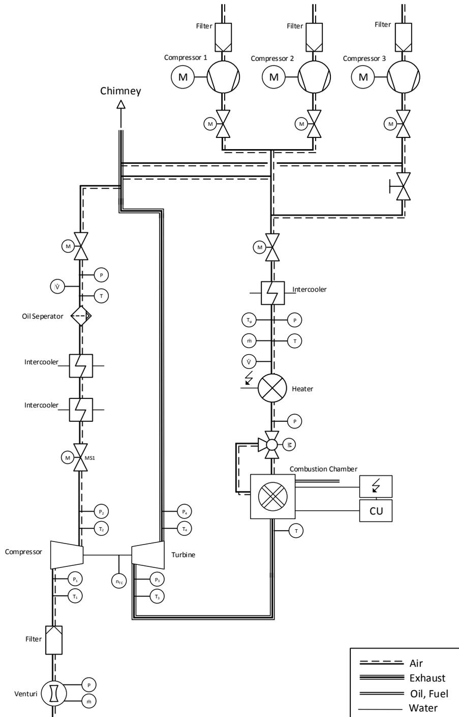
**Figure 7: Turbocharger test bench Technical University Berlin**
