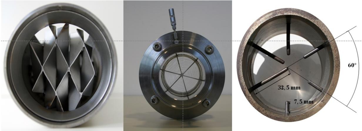
**Figure 1: Three devices to record  $T_4$ ; left: mixing device; middle: spider web sensor; right: TC ring (Baar et al. (2013))**
