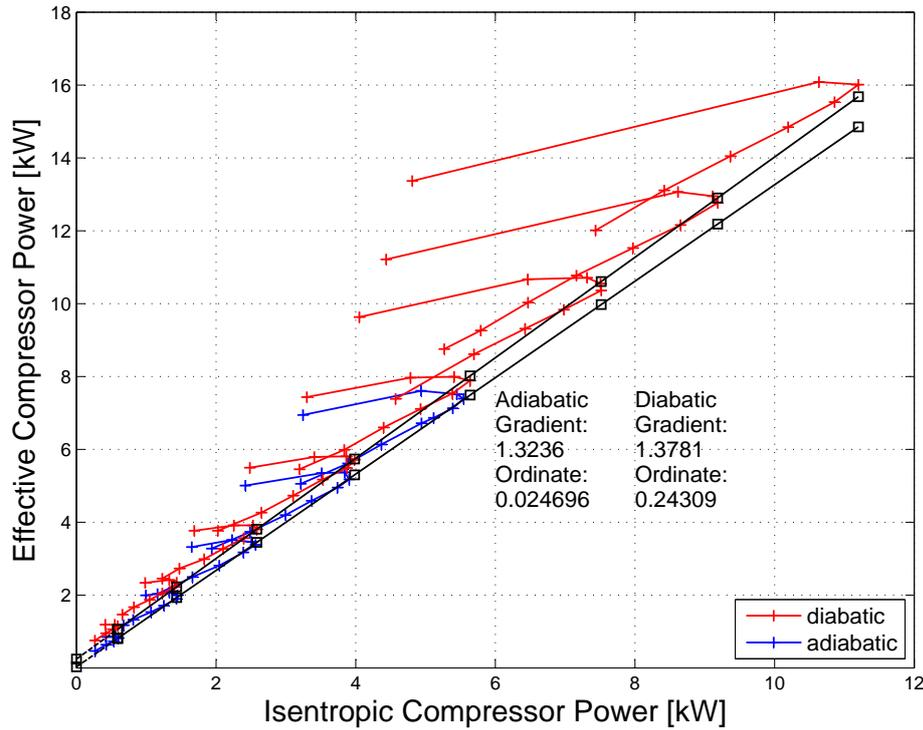
**Figure 3: Compressor power-based consideration**
