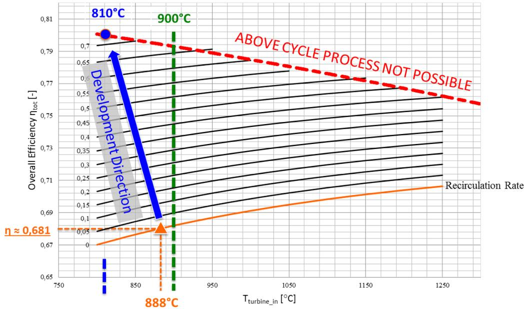
**Figure 6: Performance map of a calculated MGT-SOFC system at  $\pi = 4.5$  with the influence of the recirculation**
