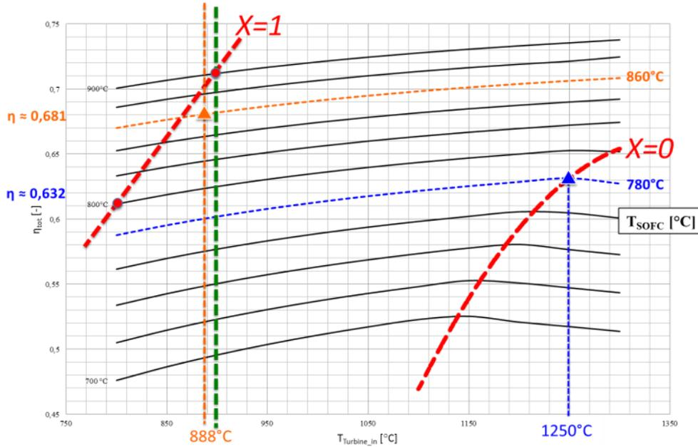
**Figure 5: Performance maps of a calculated MGT-SOFC-System at  $\pi = 4.5$**
