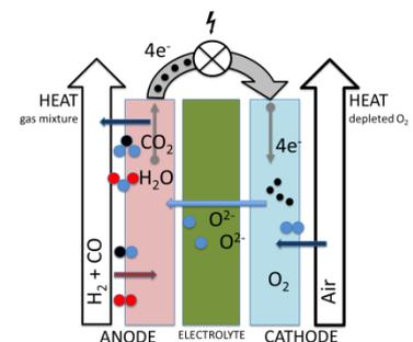
**Figure 1: Operating principle of a solid oxide fuel cell**
