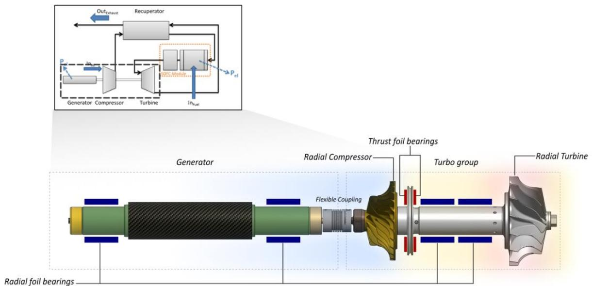
**Figure 8: General configuration of the micro gas turbine unit with foil bearings**
