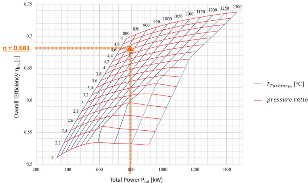
**Figure 7: Performance map of a calculated MGT-SOFC system with the influence of the pressure ratio (mapping by use of a conventional MGT100 turbo set)**
