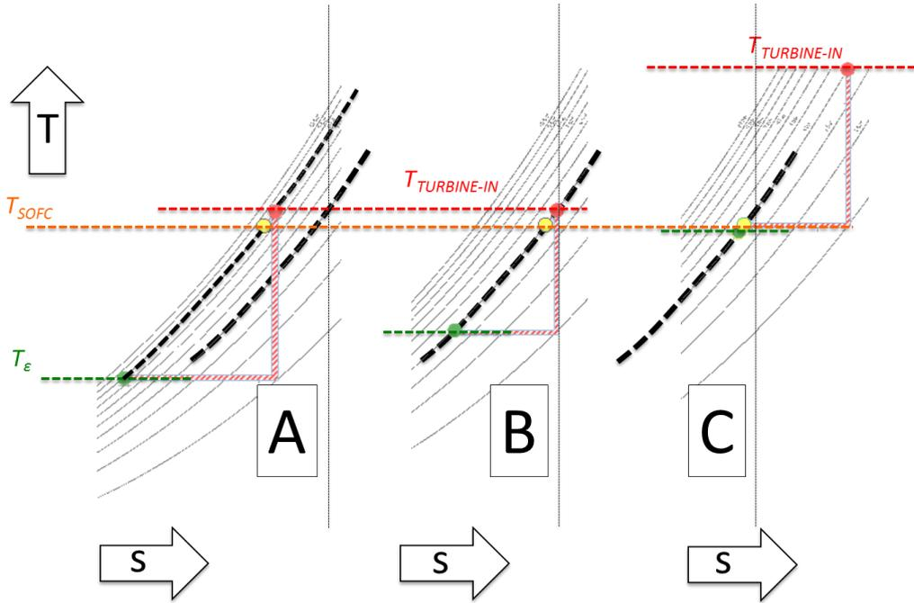
**Figure 4: Simplified examples for explanation (Boundary conditions:  $T_{SOFC} = const.$ ,  $\pi_A > \pi_B = \pi_C$ ,  $T_{Turbine\,in}^C > T_{Turbine\,in}^A = T_{Turbine\,in}^B$ )**
