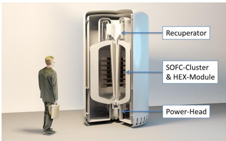
**Figure 3: Model of a future technical realisation (270 kW<sub>el</sub>)**
