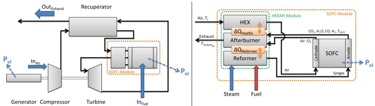
**Figure 2: Scheme of MGT-SOFC hybrid system (reforming and water-steam cycle not shown) [left] and Scheme of the SOFC-module with reformer, afterburner and HEX (without the overlaid water-steam cycle) [right]**
