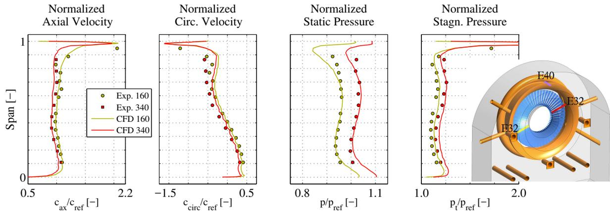
Figure 5: Comparison of CFD with measurement in plane E32
