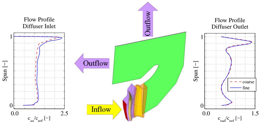
Figure 4: **Influence of blade passage mesh on diffuser flow prediction**
