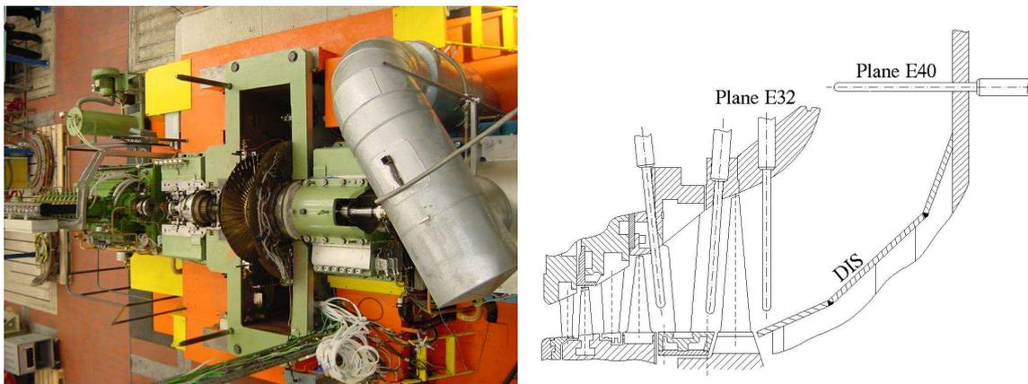
Figure 1: Image and longitudinal section of model turbine
