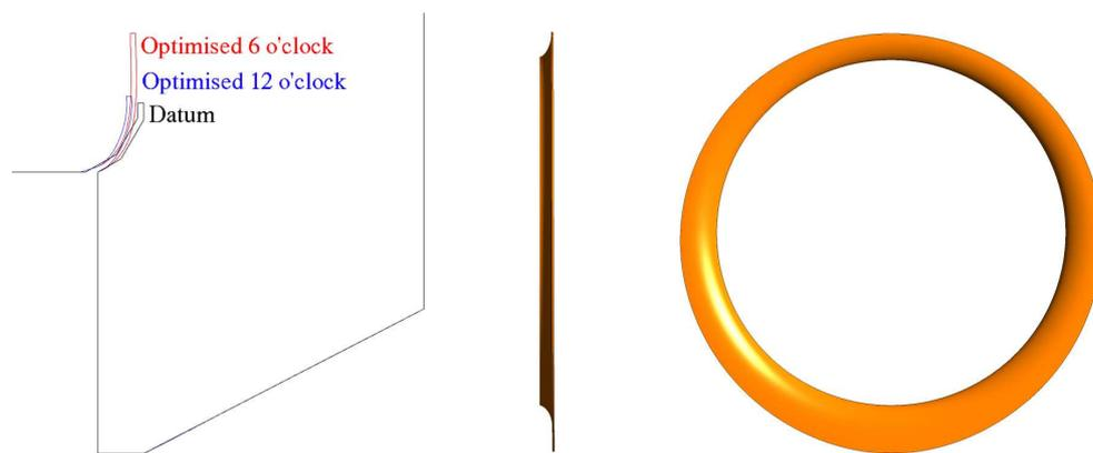
Figure 11: **Geometry of optimised diffuser shape**
