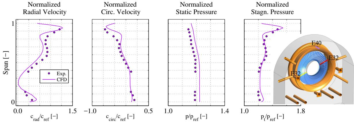
Figure 6: Comparison of CFD with measurement in plane E40
