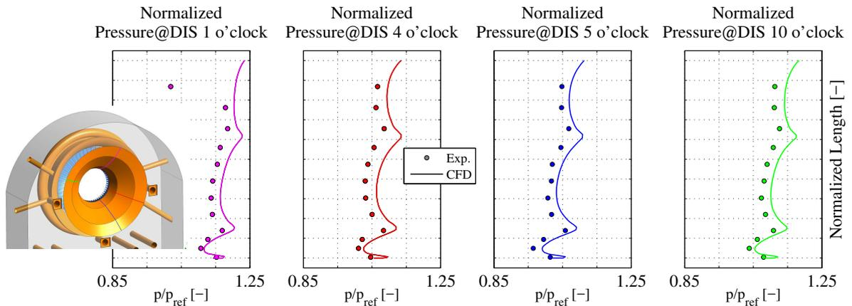
Figure 7: Comparison of CFD with measurement at diffuser inner shell
