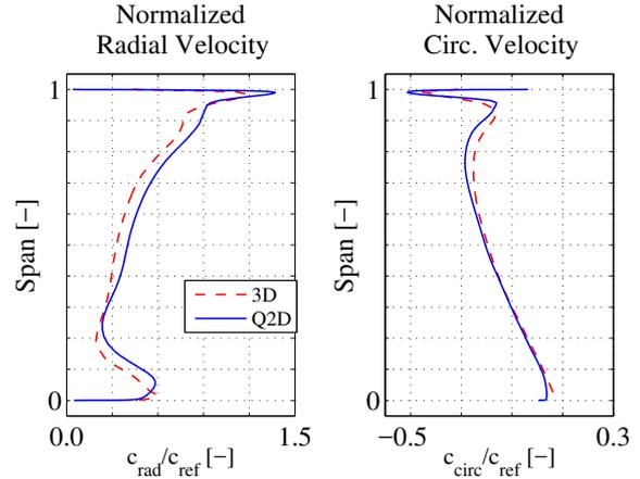
Figure 8: **Comparison of Q2D to 3D approach for 12 o'clock position**
