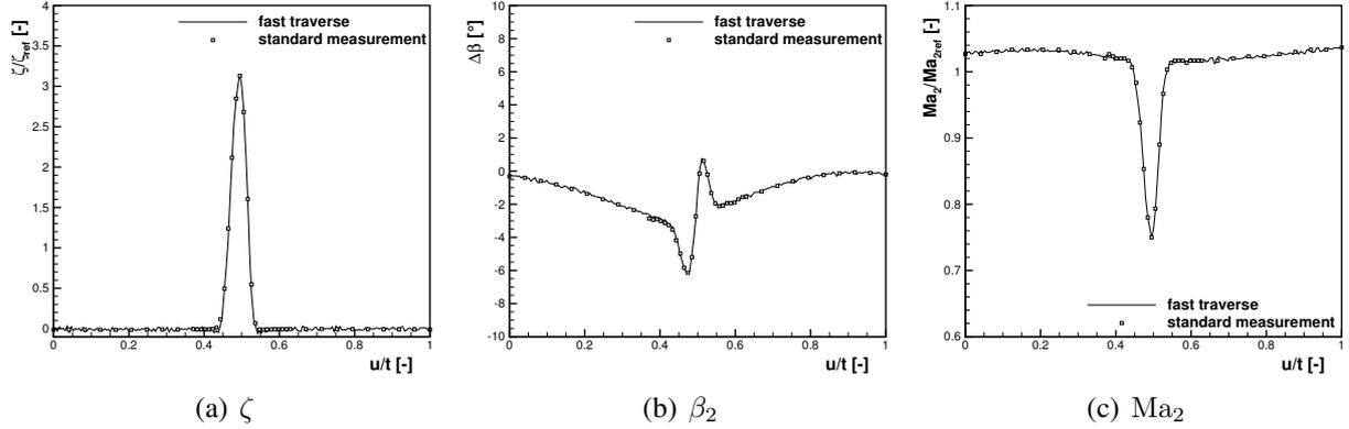
Figure 4: Flow properties measured downstream of the cascade with standard and fast traverse technique for medium Reynolds number and steady inflow
