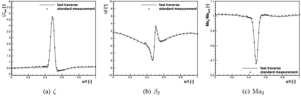
Figure 5: Flow properties measured downstream of the cascade with standard and fast traverse technique for medium Reynolds number and periodically unsteady inflow
