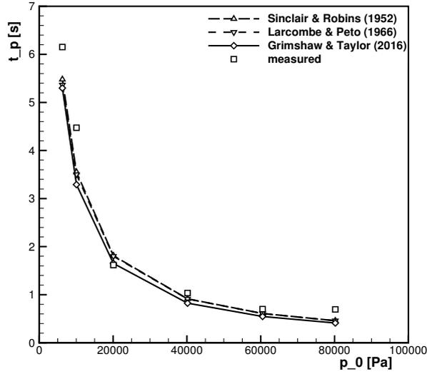
Figure 1: **Settling time as function of the initial pressure  $p_0$**
