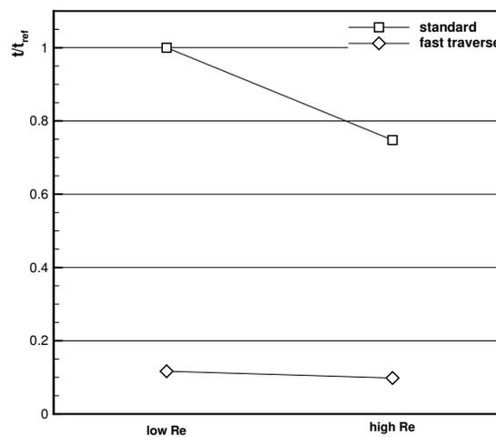
Figure 7: Total measurement time needed for a complete traverse
