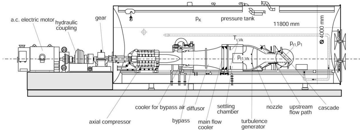
Figure 3: Drawing of the High-Speed Cascade Wind Tunnel
