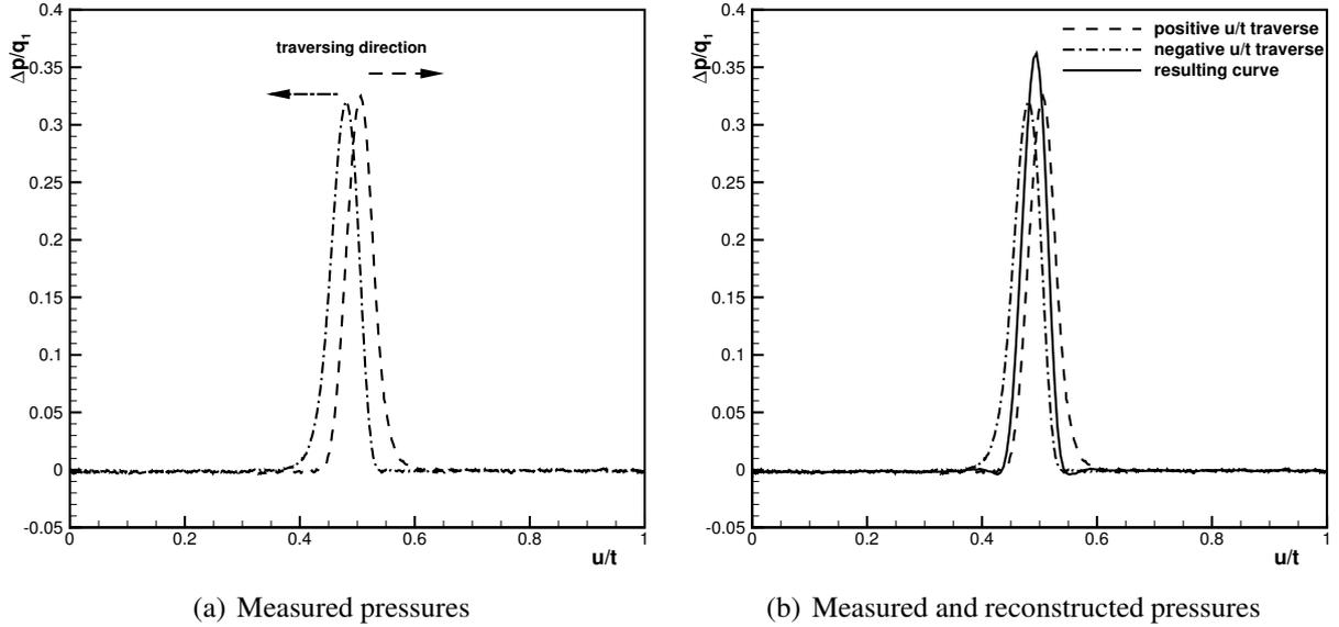
Figure 2: **Measured pressure difference between total inlet pressure and centre bore of the probe normalized by stagnation pressure and resulting normalized pressure difference as outcome of the transfer function**
