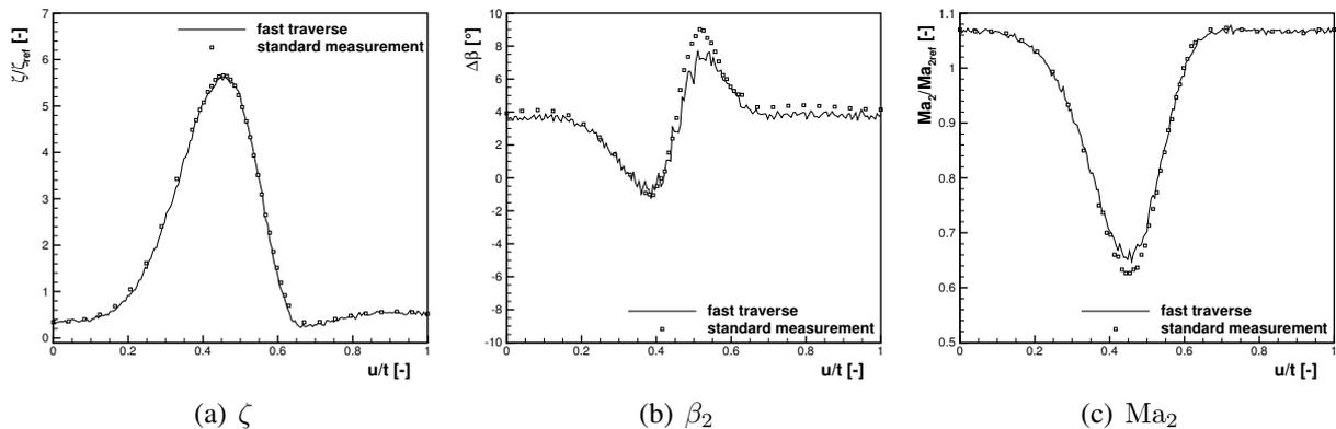
Figure 6: Flow properties measured downstream of the cascade with standard and fast traverse technique for low Reynolds number and periodically unsteady inflow
