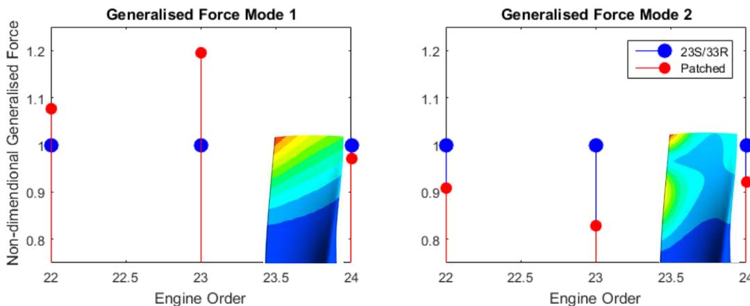
**Figure 6: Total blade generalised force for mode 1 (left) and mode 2 (right) EO**
