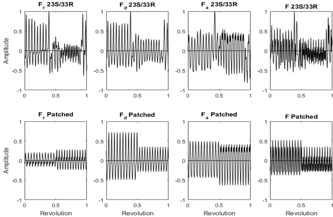
**Figure 4: Time domain total blade force for 23S/33R (top), and patched (bottom) cases**
