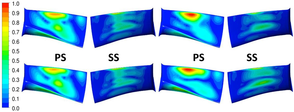
**Figure 7: Total local generalised force distribution with original (top) and patched signal (bottom) for EO22 mode 2 (left) and EO23 mode 2 (right)**
