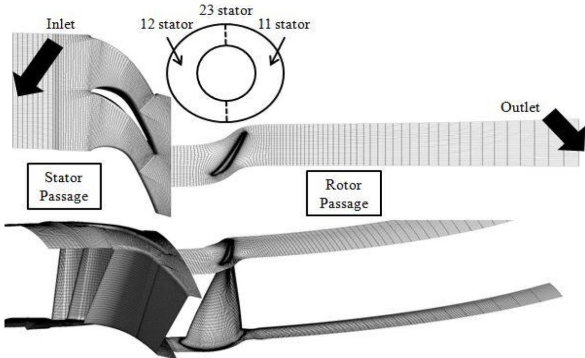
**Figure 1: Final mesh with stator passage (left) and rotor passage (right)**
