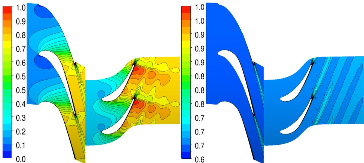
**Figure 2: Normalized Mach number (left) and entropy (right) contours on 50% span.**
