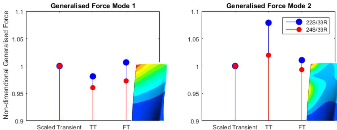
**Figure 3: Total generalised blade force with respective mode shape deflections for altered transient, time inclination (TT) and Fourier Transformation (FT) Method.**
