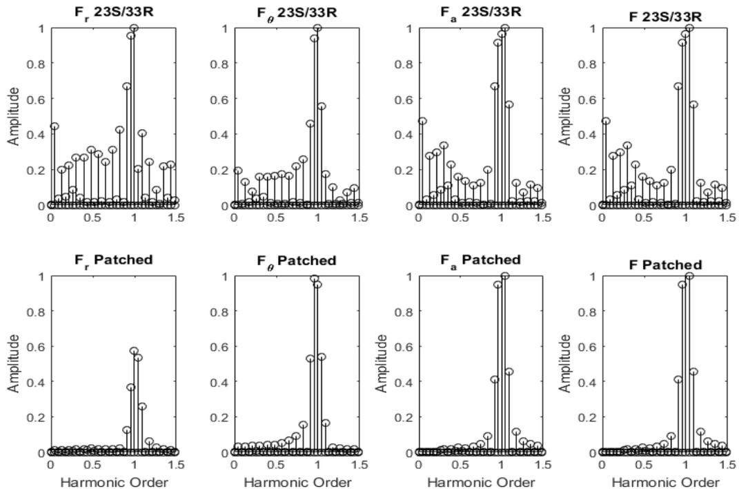
**Figure 5: Frequency domain total blade force for 23S/33R (top), and patched (bottom) cases**
