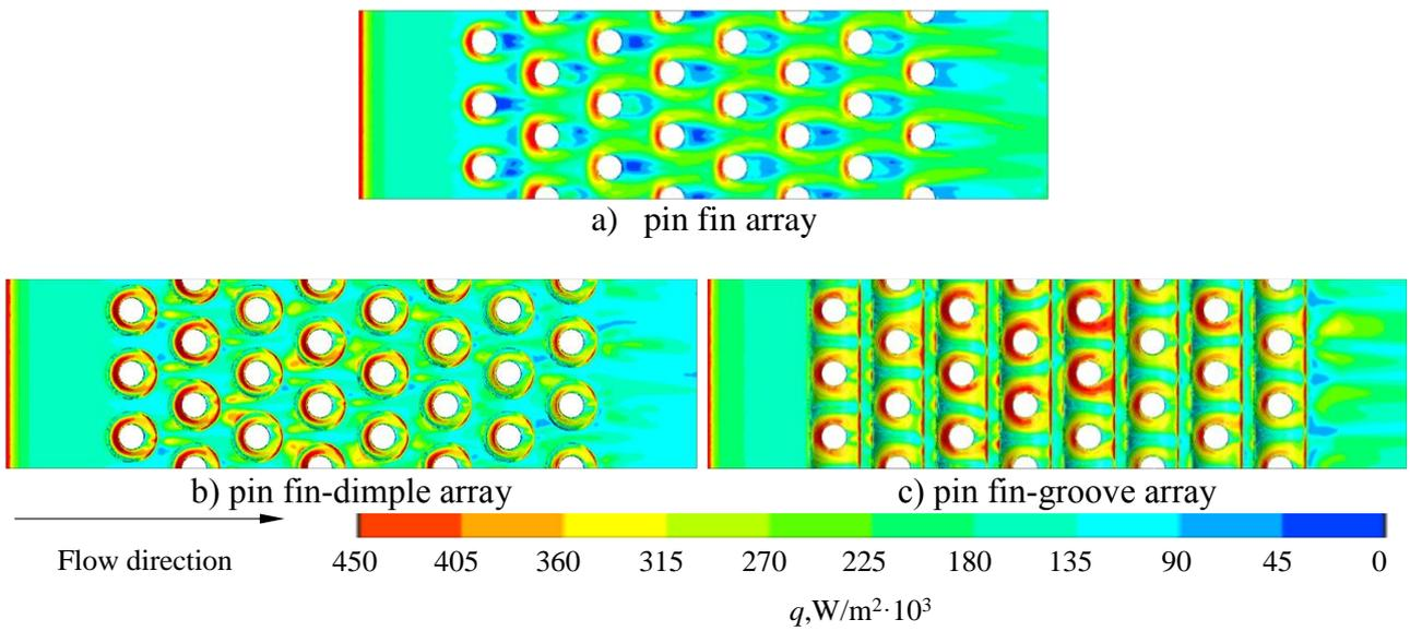
**Figure 6: Distributions of heat flux in channels with different intensifier types, Re=40000**
