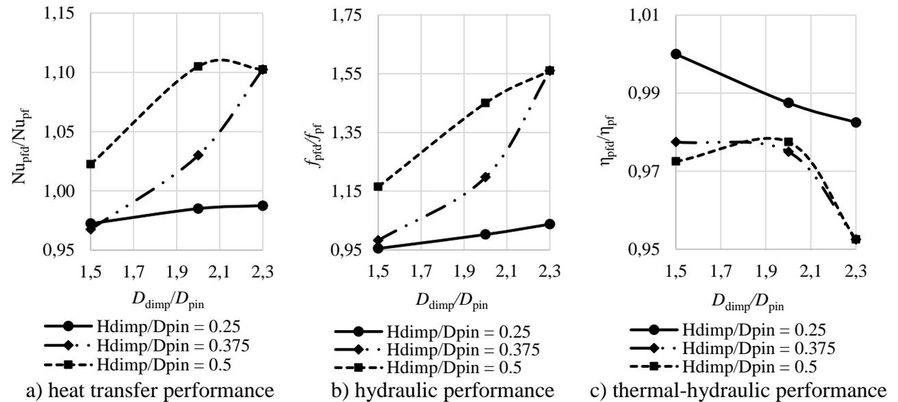
Figure 3: Influence of pin fin-dimple geometry parameters upon the channel thermal-hydraulic performance (numerical modeling results)
