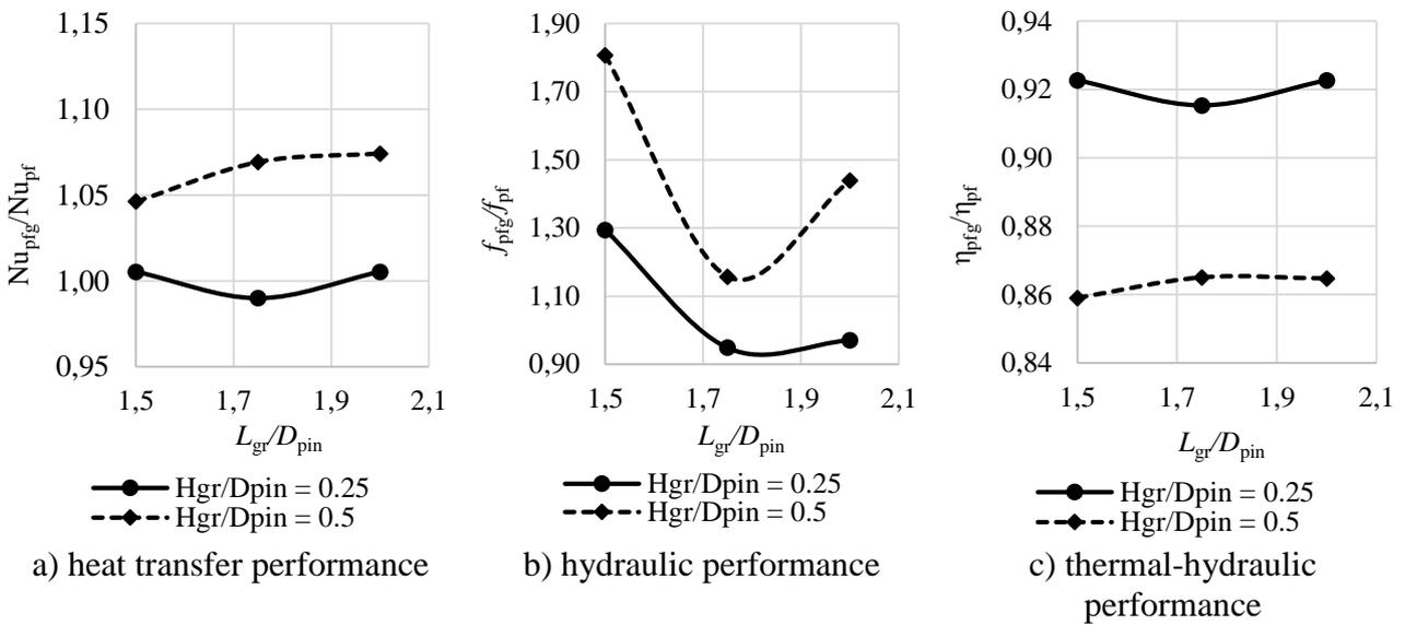
**Figure 4: Influence of pin fin-groove geometry parameters upon the channel thermal-hydraulic performance (numerical modeling results)**
