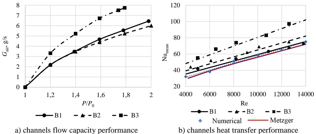
**Figure 7: The results of experimental investigation of the cooling channels with different flow turbulators (B1, B2 and B3 – experimental results for models B1, B2 and B3, Numerical – numerical results for model B1, Metzger – experimental results provided in (Metzger et. al, 1982) for model B1)**
