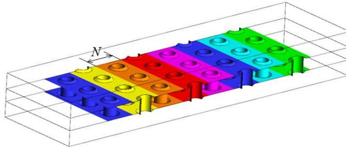
**Figure 2: The channel internal surface split into plates**
