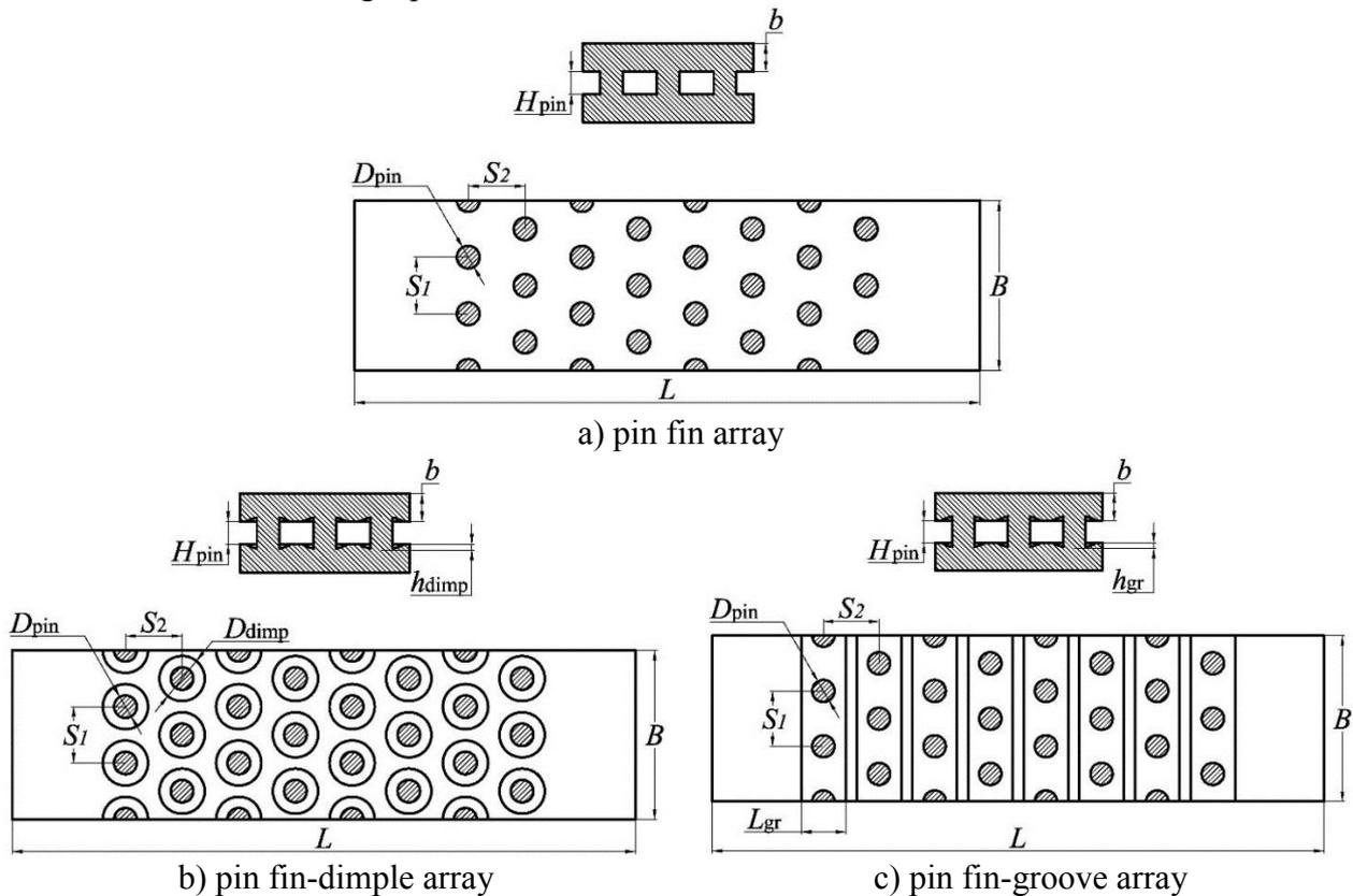
**Figure 1: Cooled channels with staggered arrays of flow turbulators**
