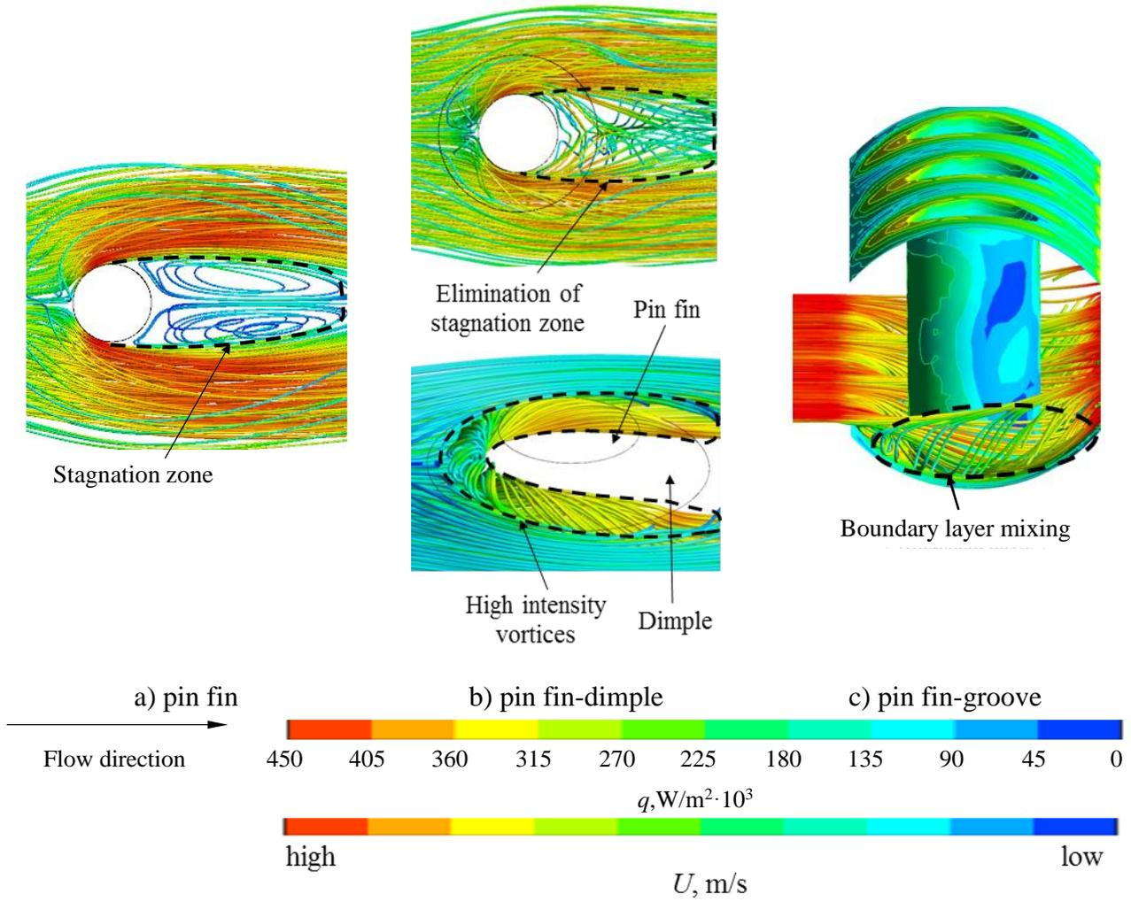
**Figure 5: Streamlines around different turbulators**
