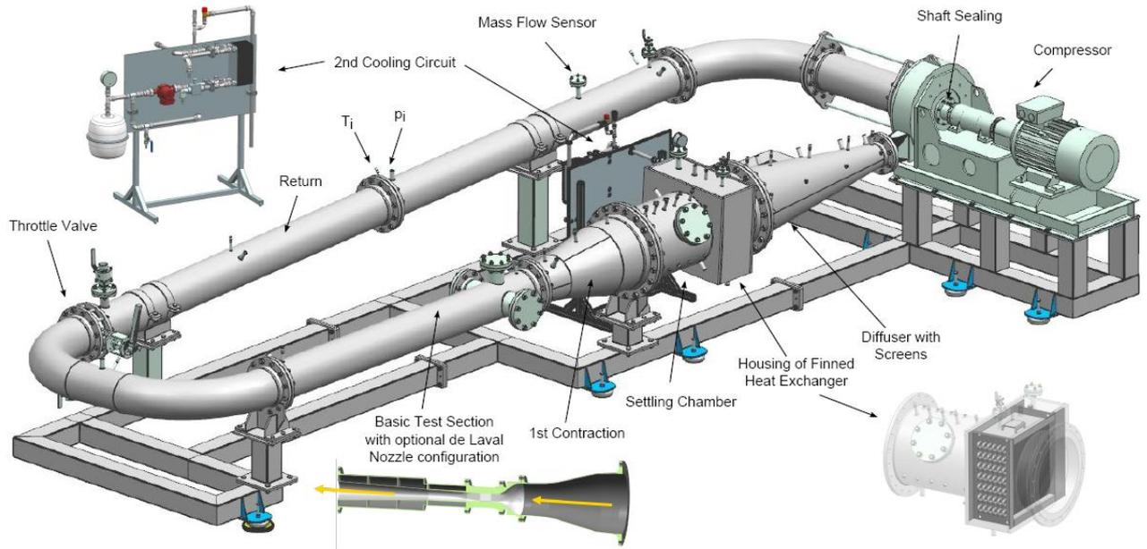
**Figure 1: Test facility CLOWT and main components (after Reinker et al. (2018))**
