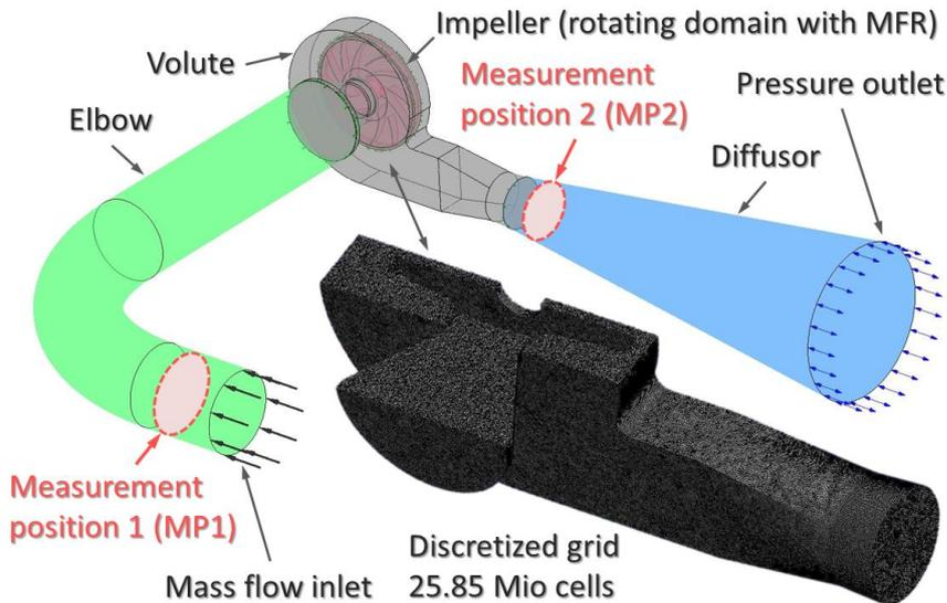
**Figure 3: Meshed fluid domain with boundary conditions**
