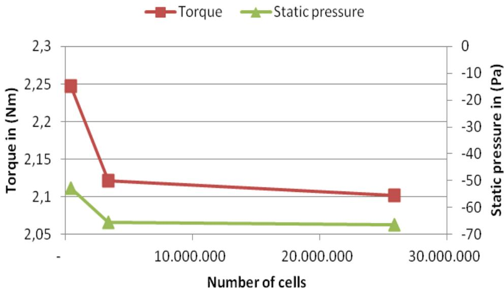
**Figure 4: Grid study for two typical fan performance quantities**
