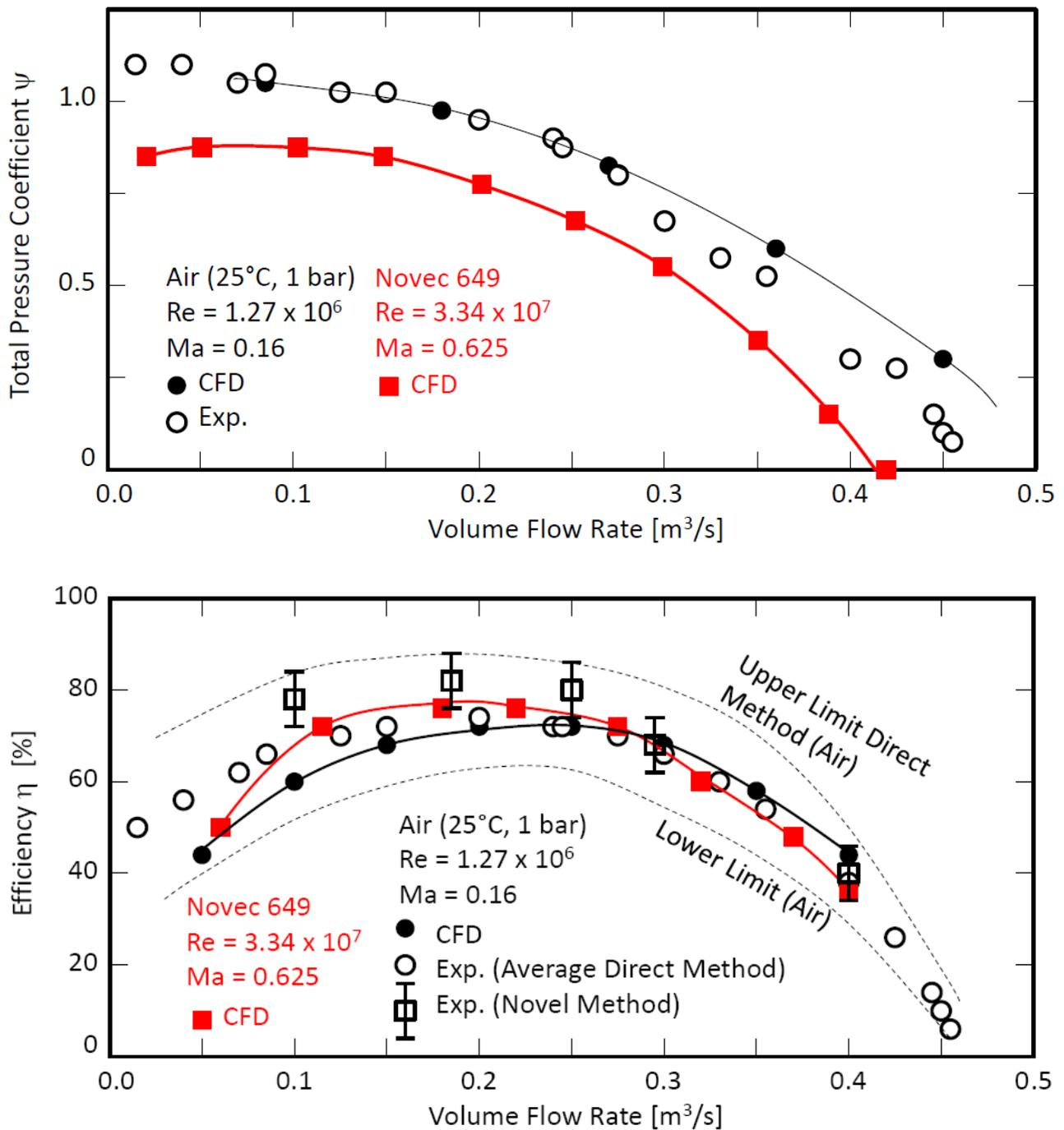
**Figure 6: Performance curve (top) and efficiency (bottom) against volume flow rate for the considered fan working with atmospheric air and Novec 649 at nominal speed (3000 rpm)**
