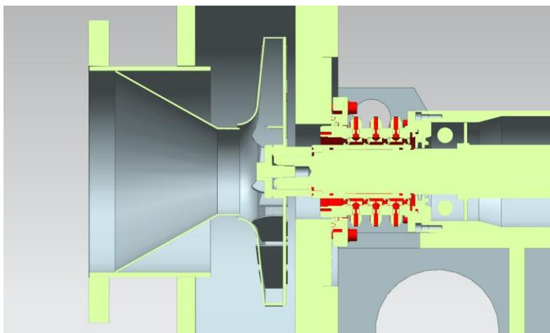
**Figure 2: Considered fan with multiple dynamic lip seal system (indicated by red color)**
