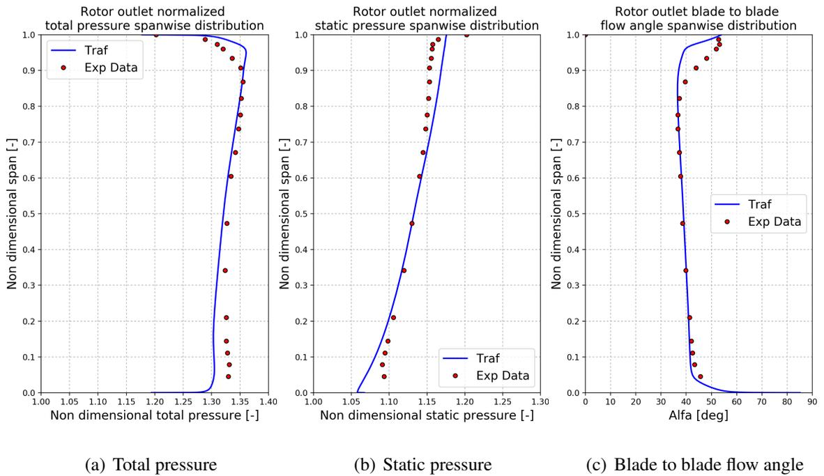
Figure 6: Rotor outlet non-dimensional spanwise distributions
