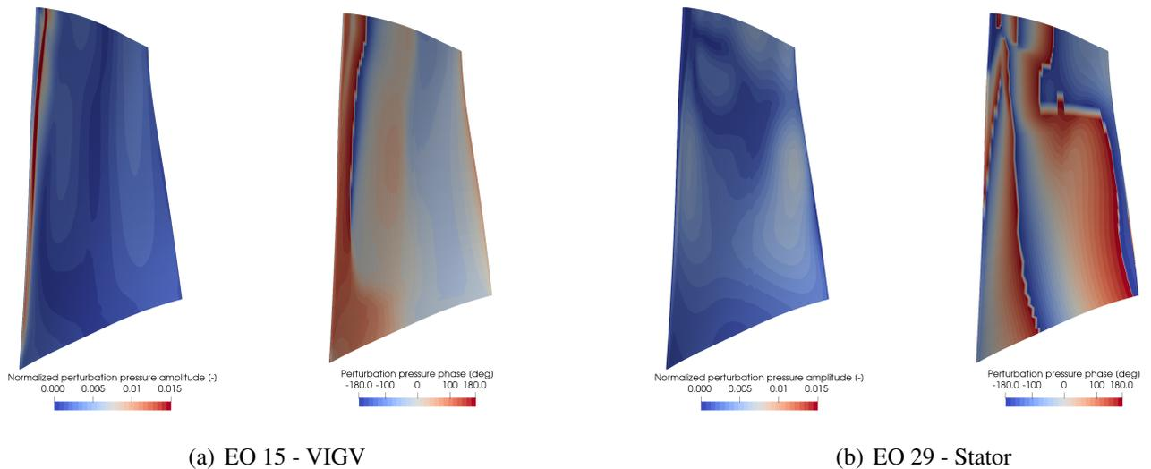
Figure 8: **Amplitude and phase of unsteady pressure harmonics**
