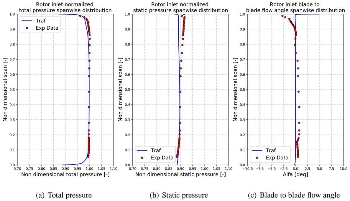
Figure 5: Rotor inlet non-dimensional spanwise distributions
