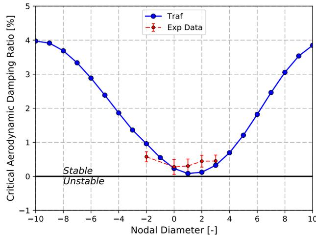
Figure 7: **Critical damping ratio vs. nodal diameter for the first bending family**
