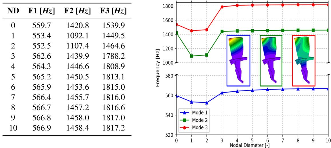
Figure 4: **Table (left) and plot (right) of blisk frequencies**
