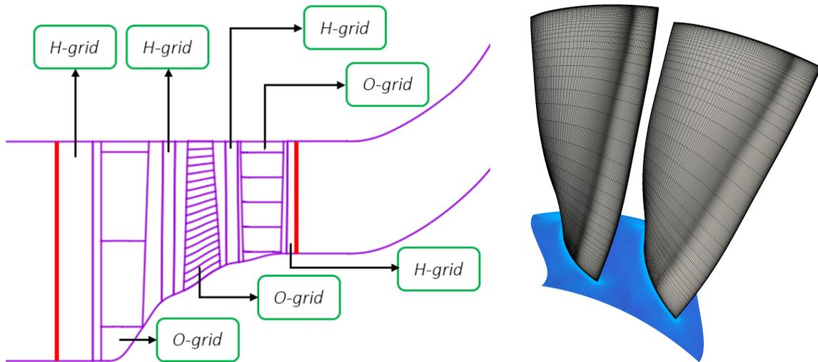
Figure 2: **Fluid domain: meridional sketch (left) and 3D rotor blade grid (right)**
