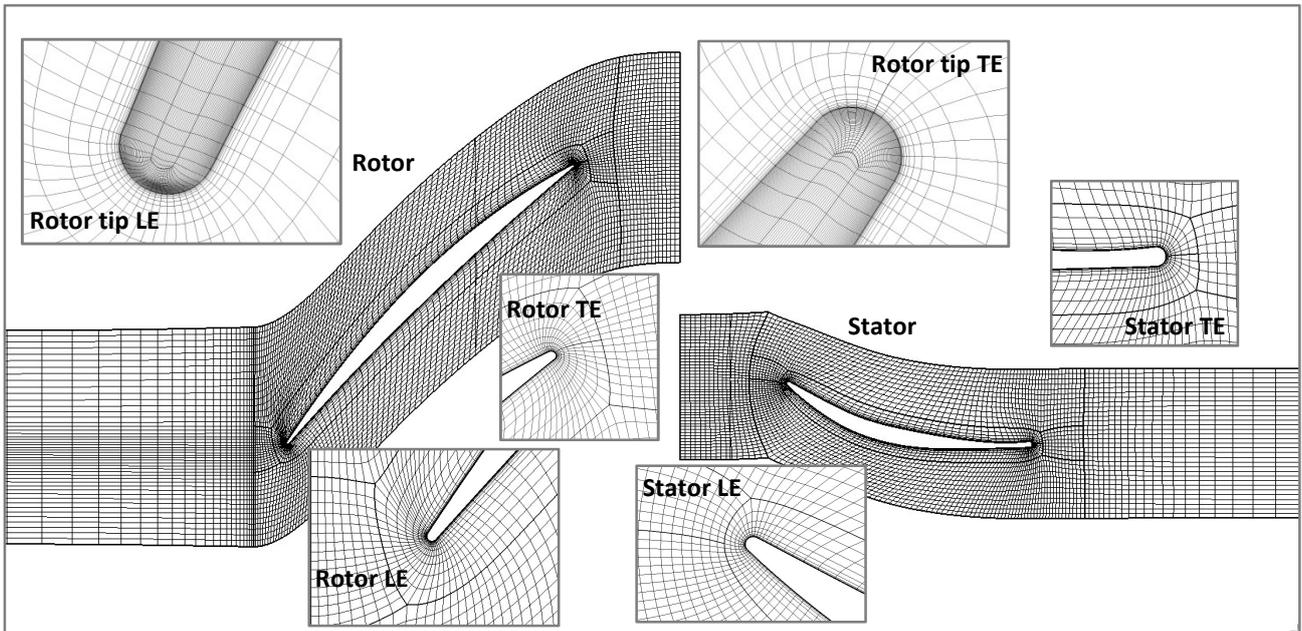
**Figure 2: Blade-to-blade mesh at mid span (coarse grid level shown)**
