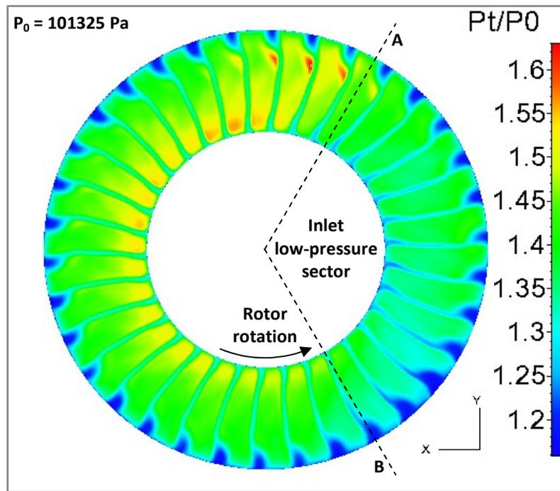
**Figure 8: Axial view of instantaneous total pressure contours at St. 3**
