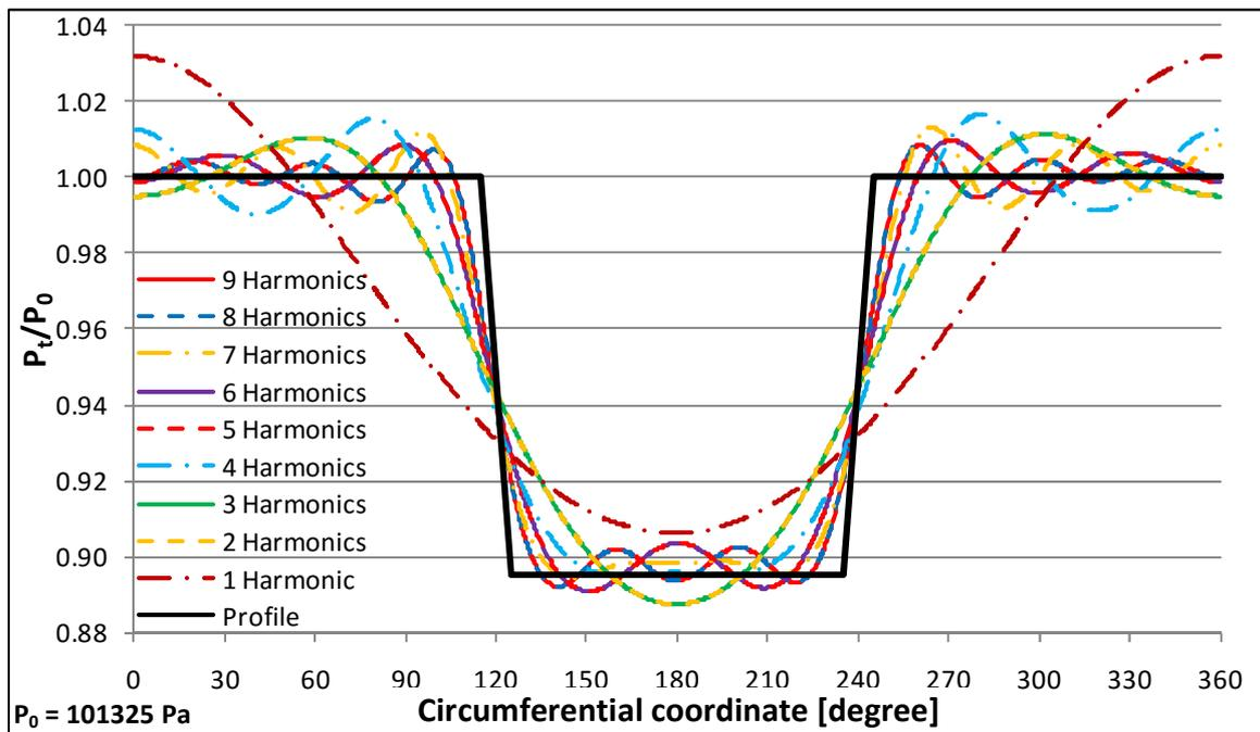
Figure 3: Inlet total pressure profile and its reconstructed harmonic representations
