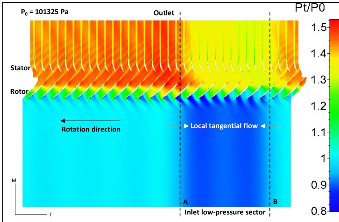
Figure 4: Mid-span blade-to-blade view of instantaneous total pressure contours
