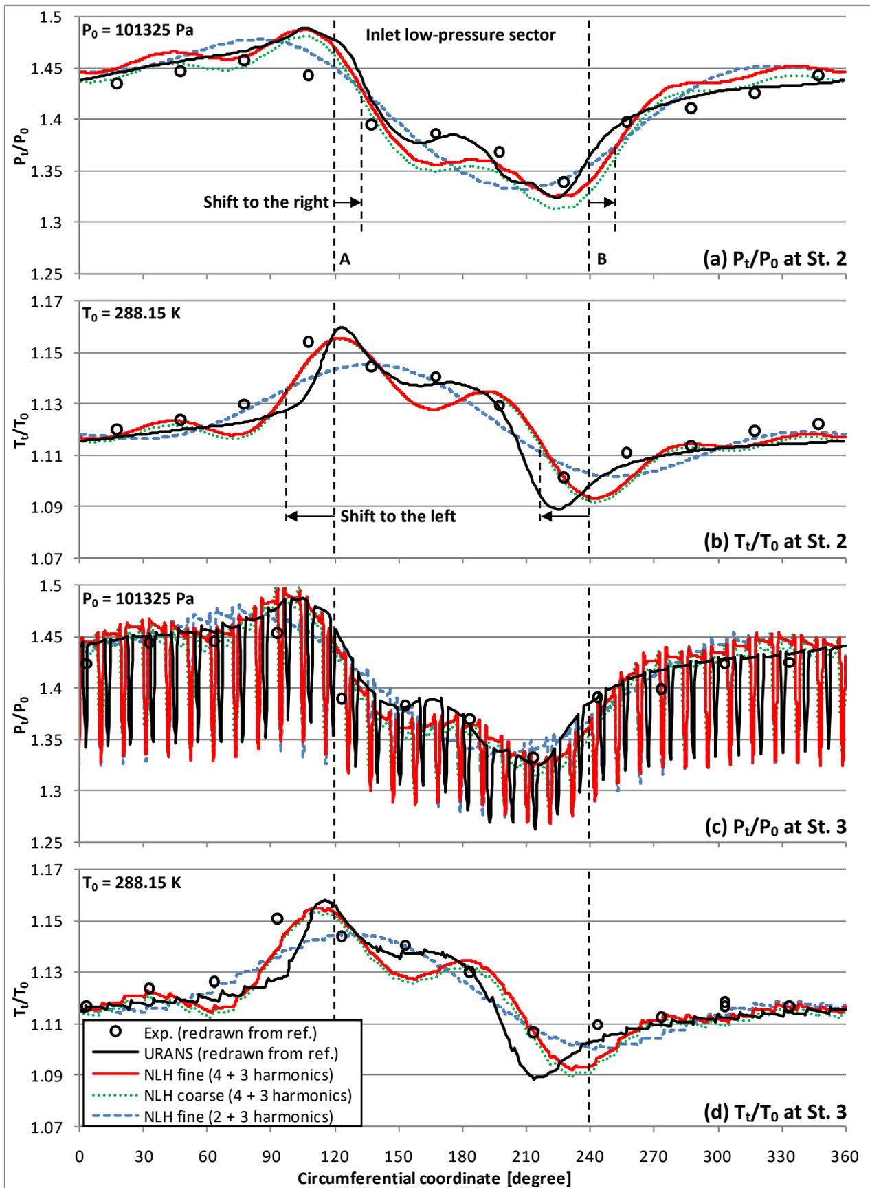
Figure 7: Mid-span time-mean total pressure and total temperature distribution at St. 2 (rotor-stator interface) and St. 3 (downstream of the stator), ref.: Jerez Fidalgo *et al.*, 2012
