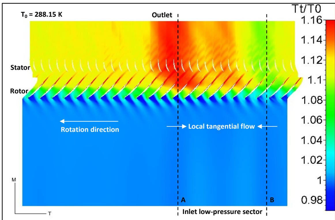
Figure 5: Mid-span blade-to-blade view of instantaneous total temperature contours
