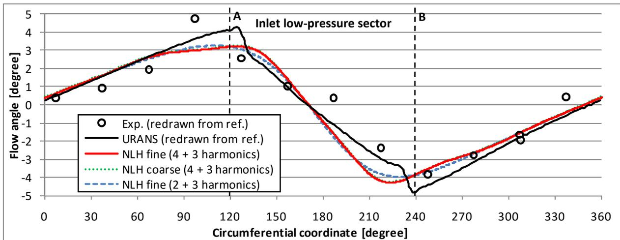
**Figure 6: Mid-span flow angle distribution at St. 1 (upstream of the rotor), ref.: Jerez Fidalgo *et al.*, 2012**
