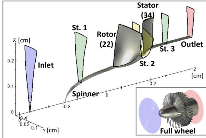
**Figure 1: Computational domain (shroud and periodic boundaries not shown)**
