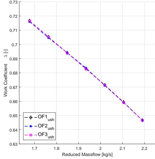
Figure 6: Work input comparison for different optimized diffusers
