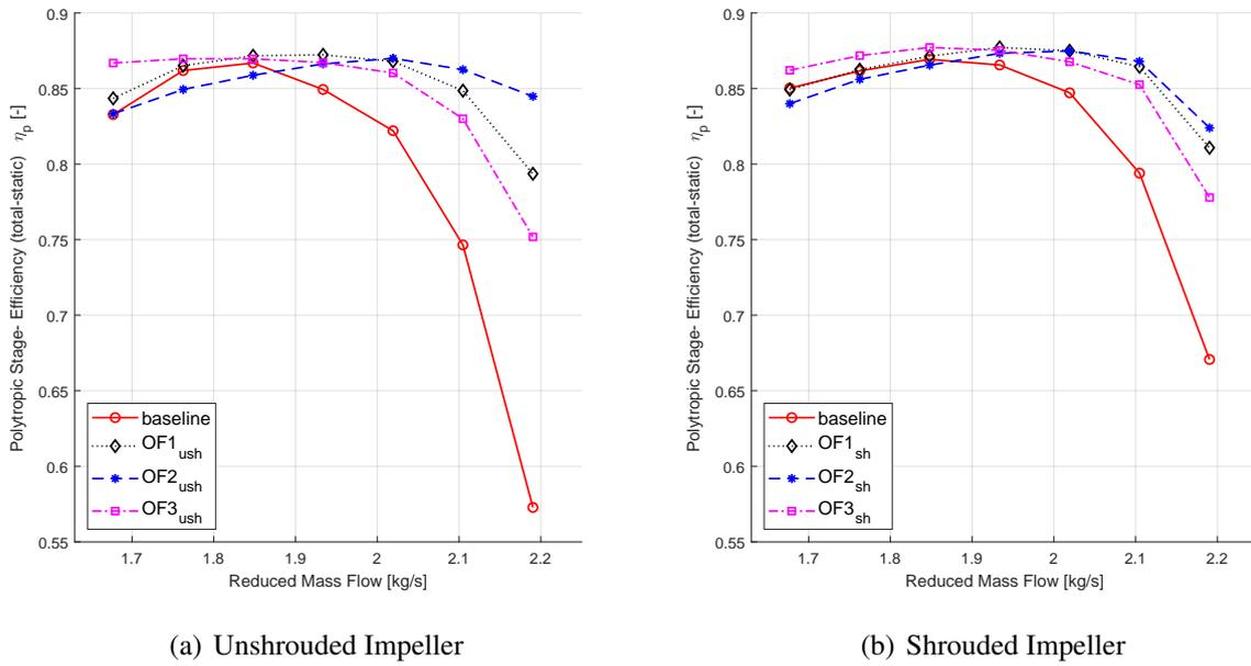
Figure 10: Polytropic stage efficiency characteristics of the differently optimized radial diffuser geometries
