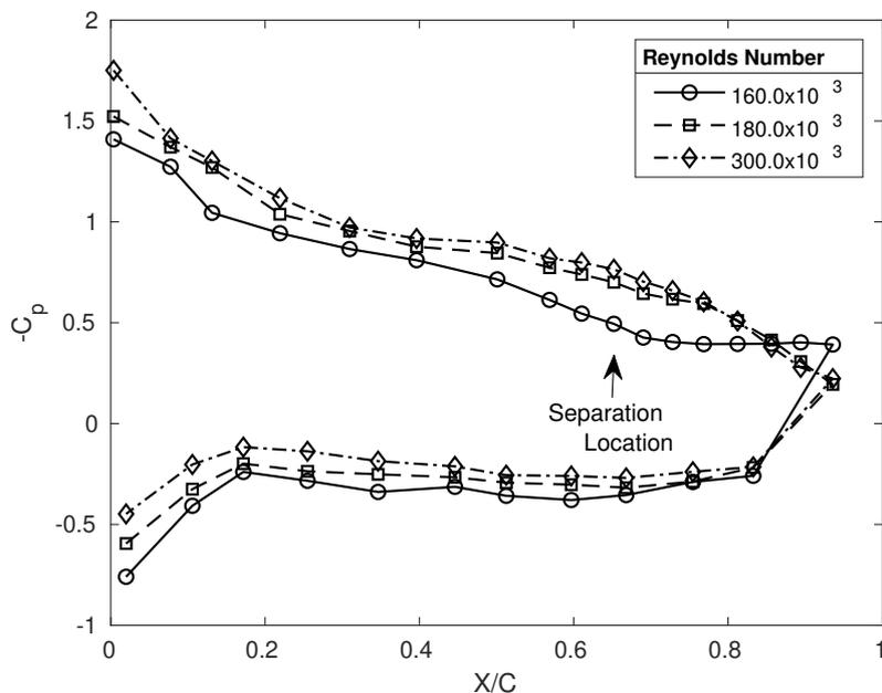
Figure 2: Pressure coefficient distribution at different Reynolds numbers
