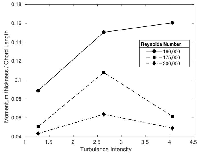
Figure 5: **Momentum thickness variation for different Reynolds numbers and turbulence intensities.**
