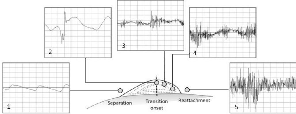
Figure 3: **Fluctuating velocity on the suction surface at  $Re = 100,000$  and incoming turbulence intensity of 1.27% (Taghavi and Etemadi, 2014)**
