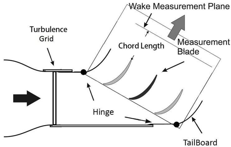
Figure 1: **Schematic view of cascade**
