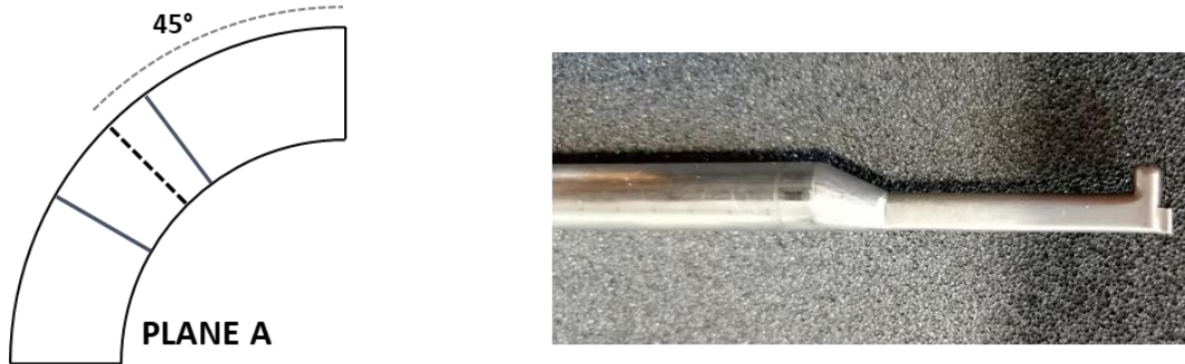
Figure 4: Detail of the five-hole-probe head and position of the measurement sectors upstream (plane A) of the LPT stage.
