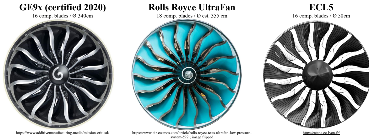
Fig. 2 Modern industrial low-speed composite fans and Open Test Case ECL5/CATANA
